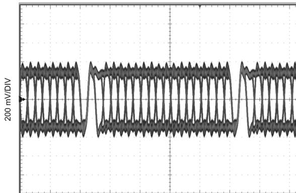
Figure 24. Serial Output Dual Mode, 50 MHz, VSEL = H, No Pre-Emphasis
