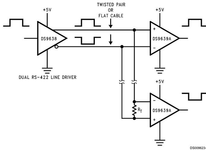
$R_T \geq 50\Omega$  for RS-422 operation.
