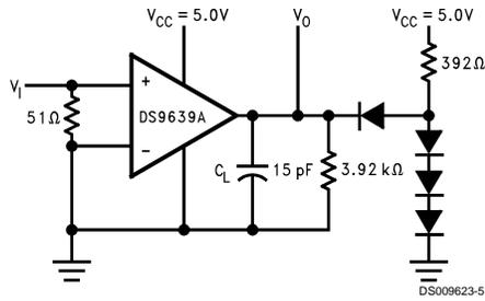
$C_L$  includes jig and probe capacitance.
