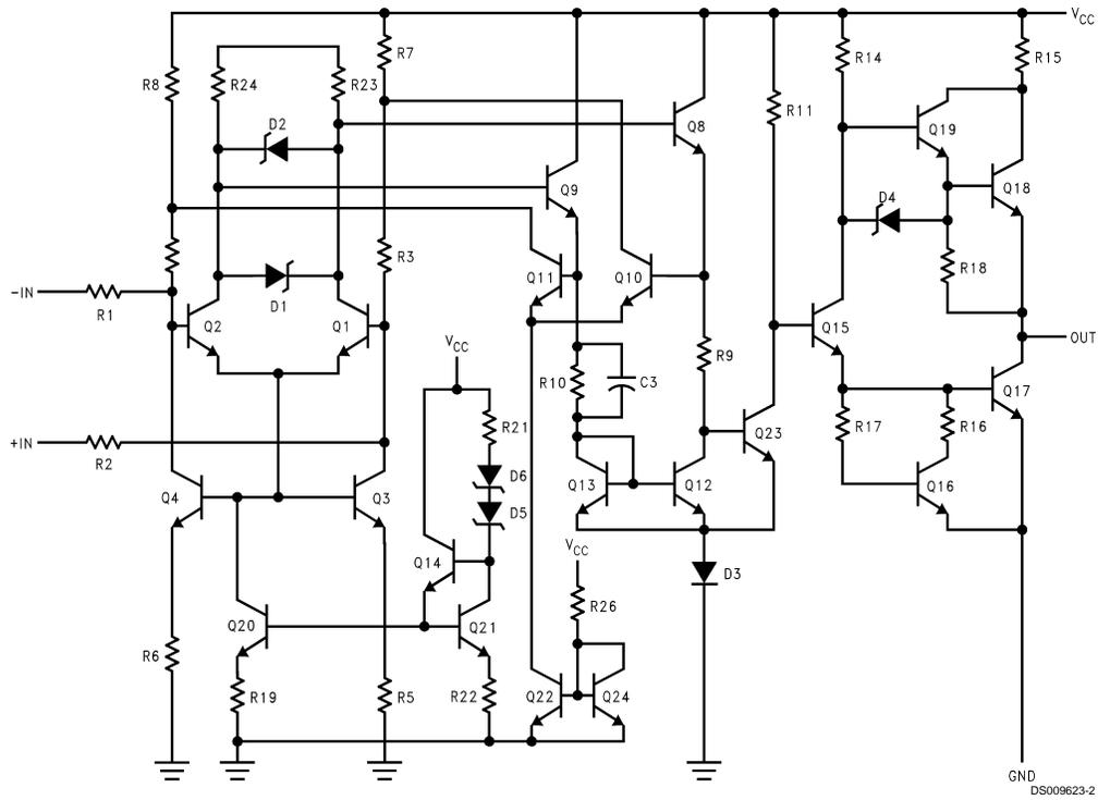
FIGURE 1. Equivalent Circuit
