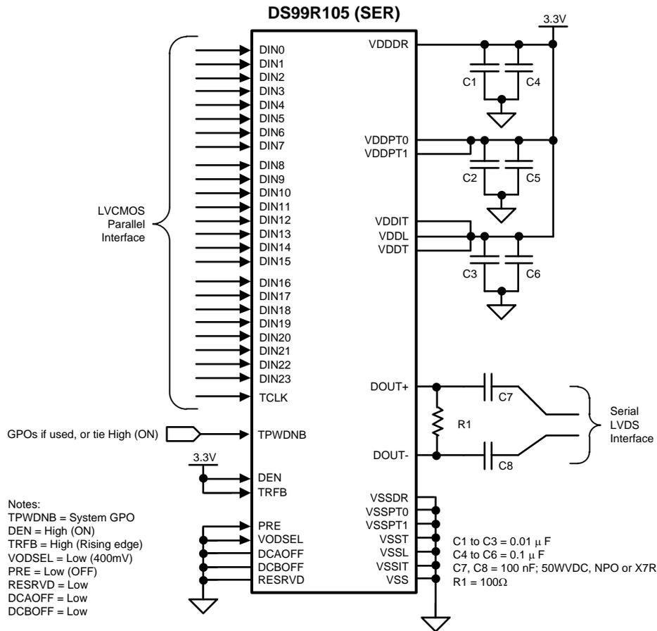
Figure 20. DS99R105 Typical Application Connection
