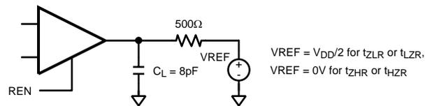
Note:  $C_L$  includes instrumentation and fixture capacitance within 6 cm of ROUT[23:0]
