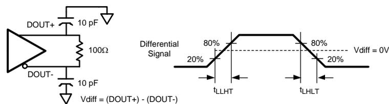
Figure 3. Serializer LVDS Output Load and Transition Times
