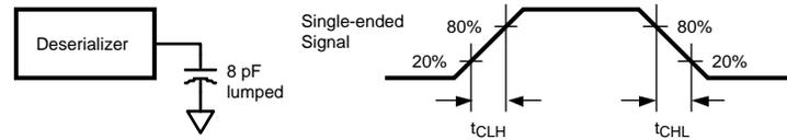
Figure 11. Deserializer LVMOS/LVTTL Output Load and Transition Times
