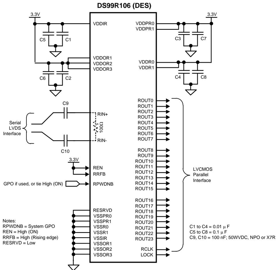
Figure 21. DS99R106 Typical Application Connection
