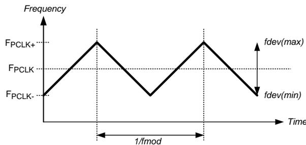
**Figure 17. SSCG Waveform**
