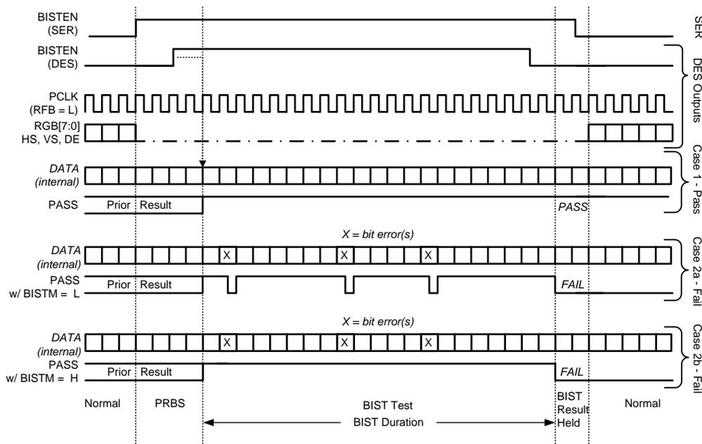
Figure 19. BIST Waveforms
