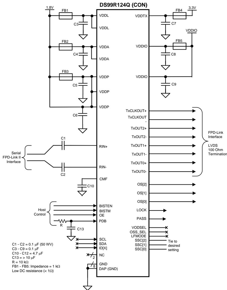
Figure 24. DS99R124Q Typical Connection Diagram — Pin Control
