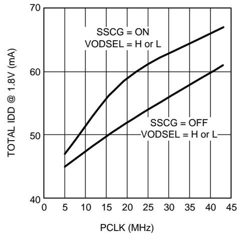
Figure 13. Typical Total IDD Current (1.8V Supply) as a Function of PCLK
