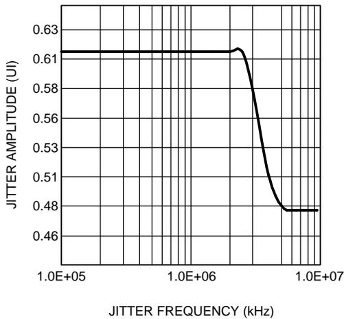
Figure 12. Typical Input Jitter Tolerance Curve at 43 MHz
