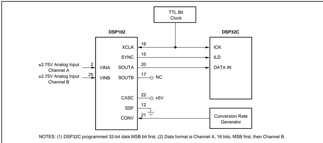
FIGURE 21. Using DSP102 with DSP32C in Cascade Mode.
