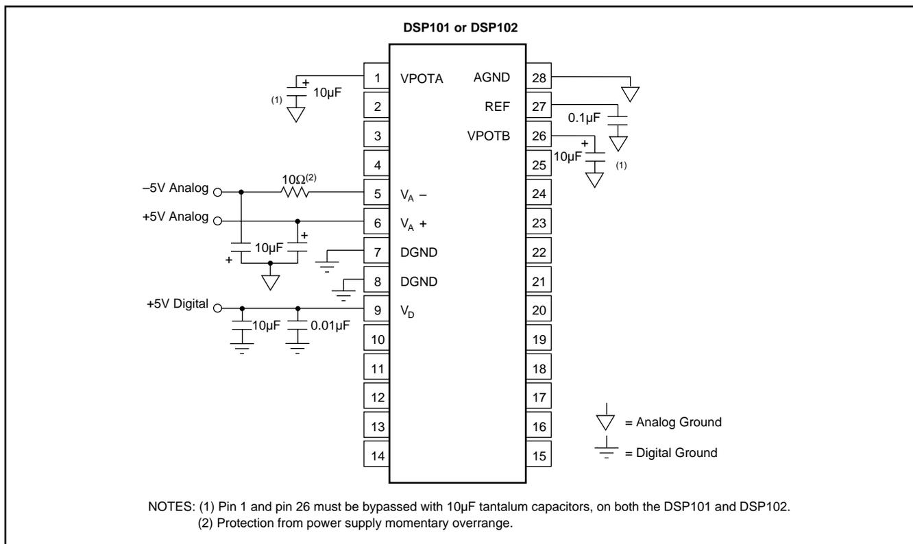
FIGURE 6. DSP101 or DSP102 Power Supply Connections.
