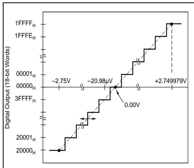
FIGURE 3. Analog Input to Digital Output Diagram.
