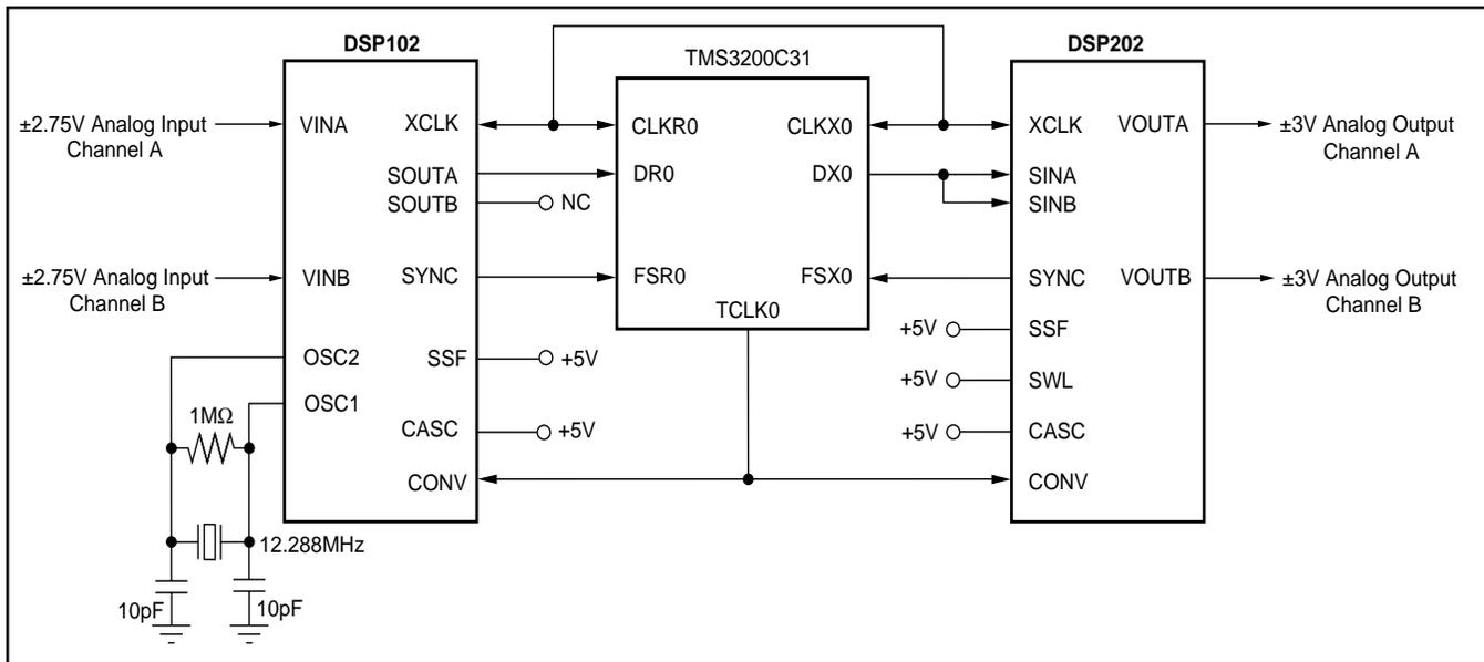
FIGURE 17. Two Channel Analog I/O Using TMS320C31.
