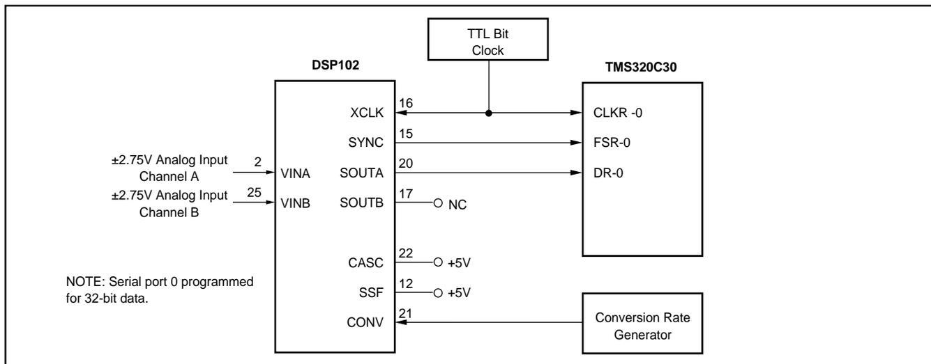
FIGURE 13. Using DSP102 with TMS320C30 in Cascade Mode.
