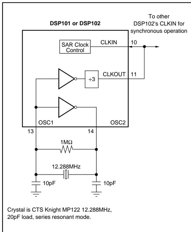
FIGURE 5. DSP101 or DSP102 Conversion Clock Circuit.
