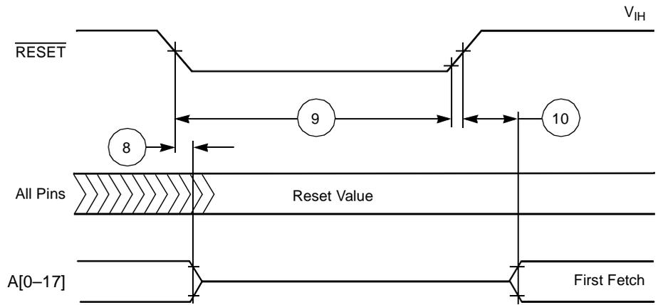
Figure 2-3. Reset Timing
