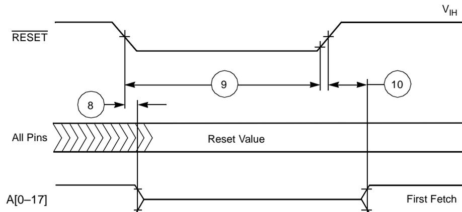
**Figure 2-3.** Reset Timing
