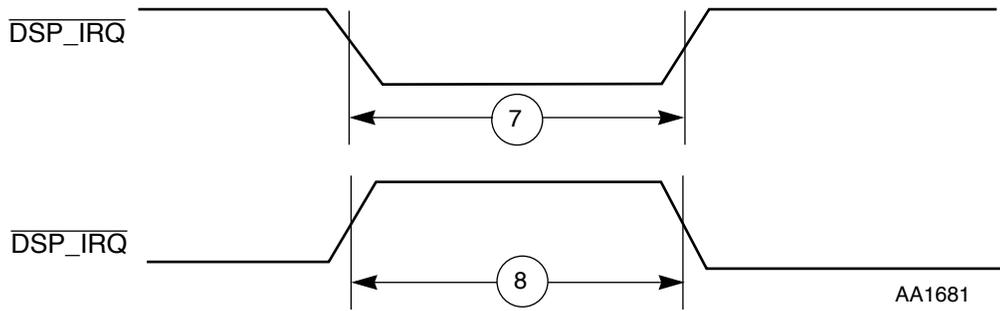
**Figure 2-3 DSP External Interrupt Timing (Negative Edge-Triggered)**
