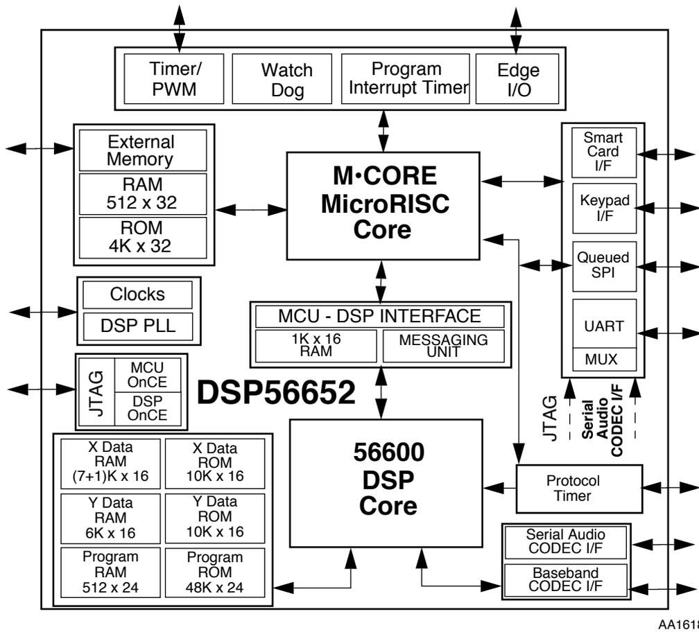
**Figure 1-1 DSP56652 System Block Diagram**
