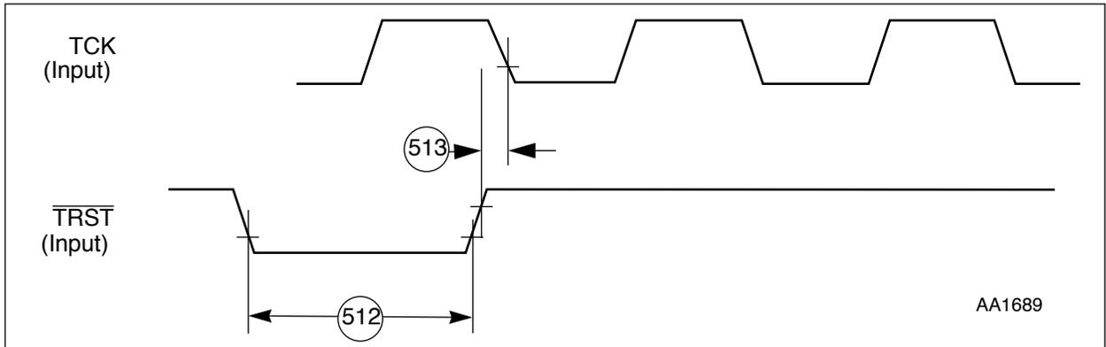
Figure 2-13 TRST Timing Diagram
