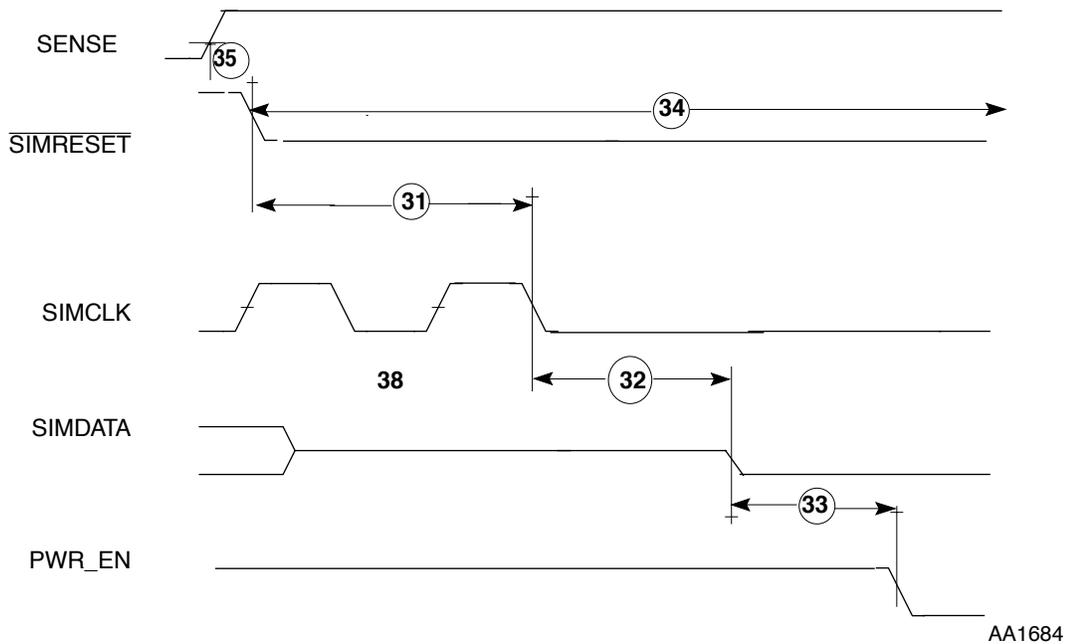
Figure 2-6 Smart Card Interface Power Down AC Timing
