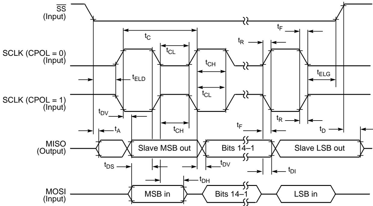
Figure 21. SPI Slave Timing (CPHA = 1)
