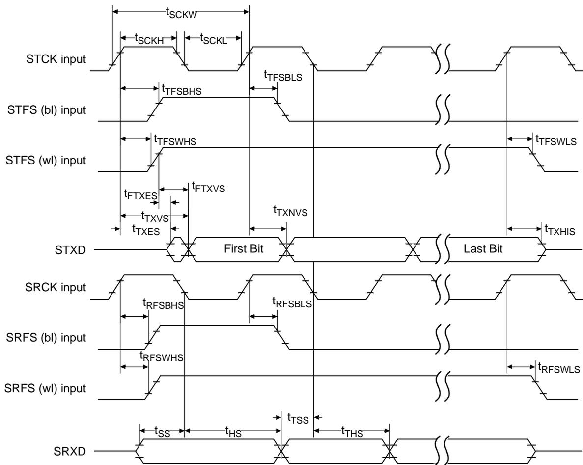
Figure 24. Slave Mode Clock Timing
