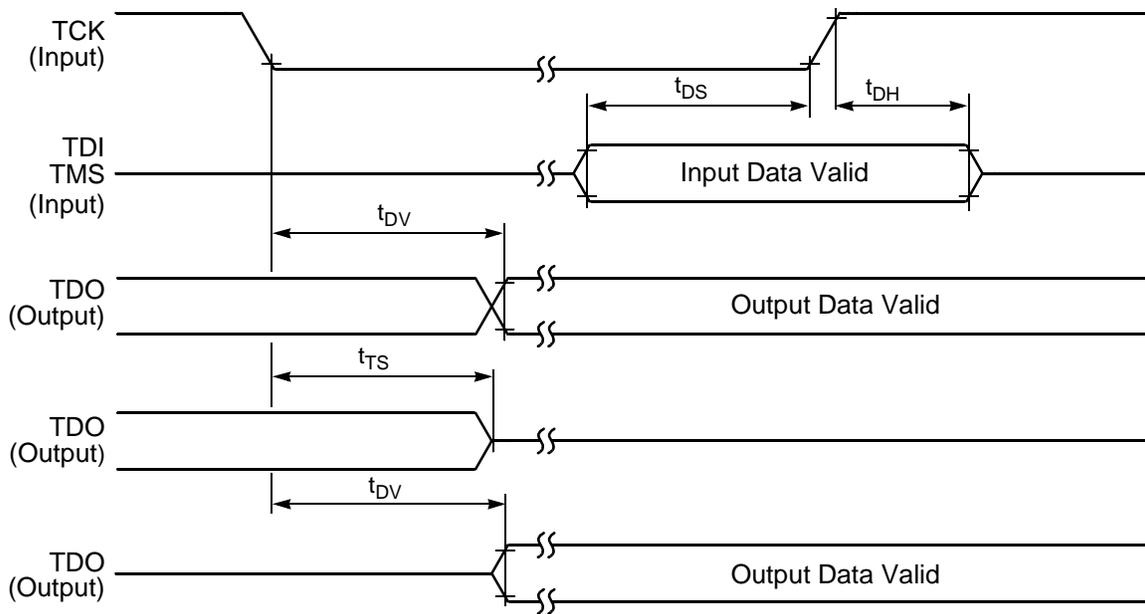
Figure 29. Test Access Port Timing Diagram
