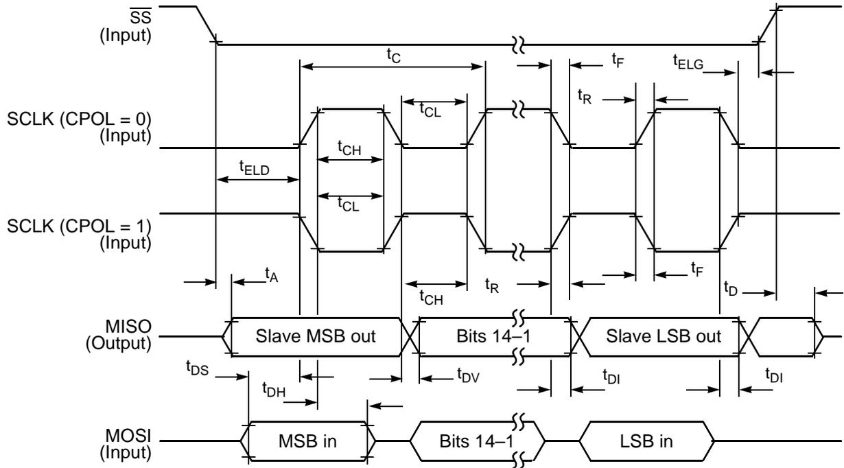
Figure 20. SPI Slave Timing (CPHA = 0)
