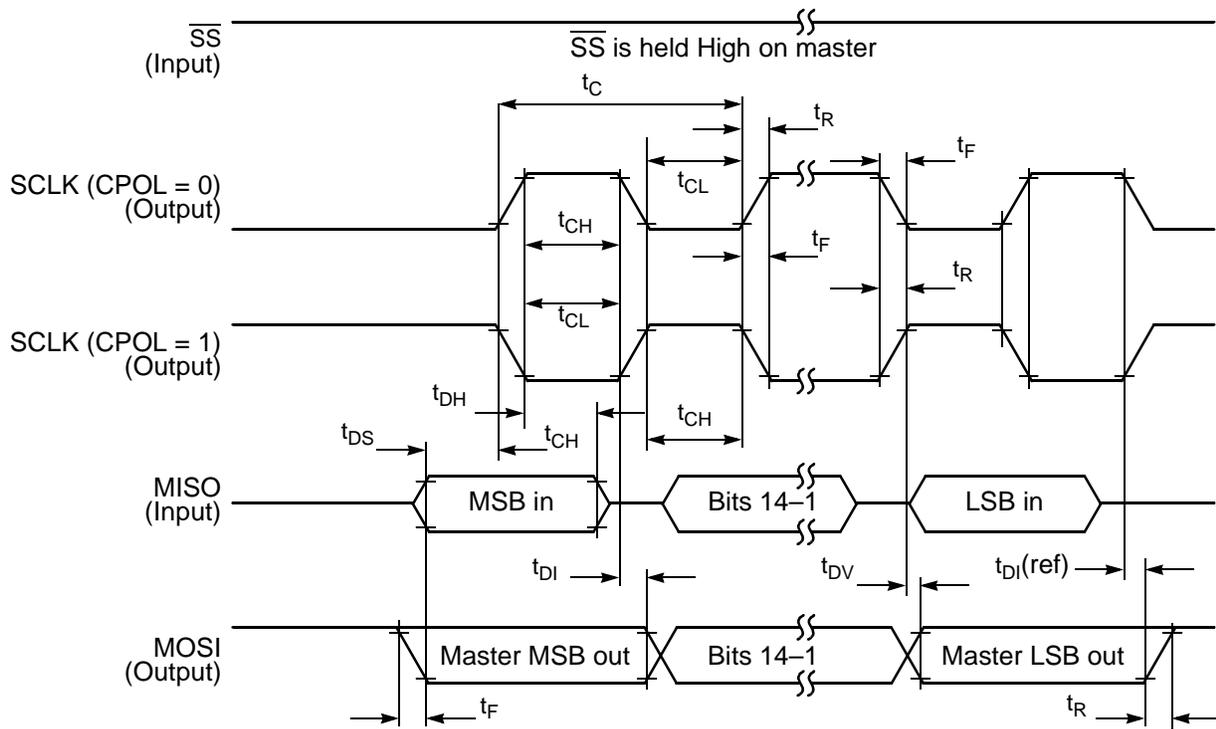
**Figure 18. SPI Master Timing (CPHA = 0)**
