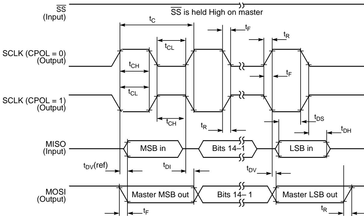
**Figure 19. SPI Master Timing (CPHA = 1)**
