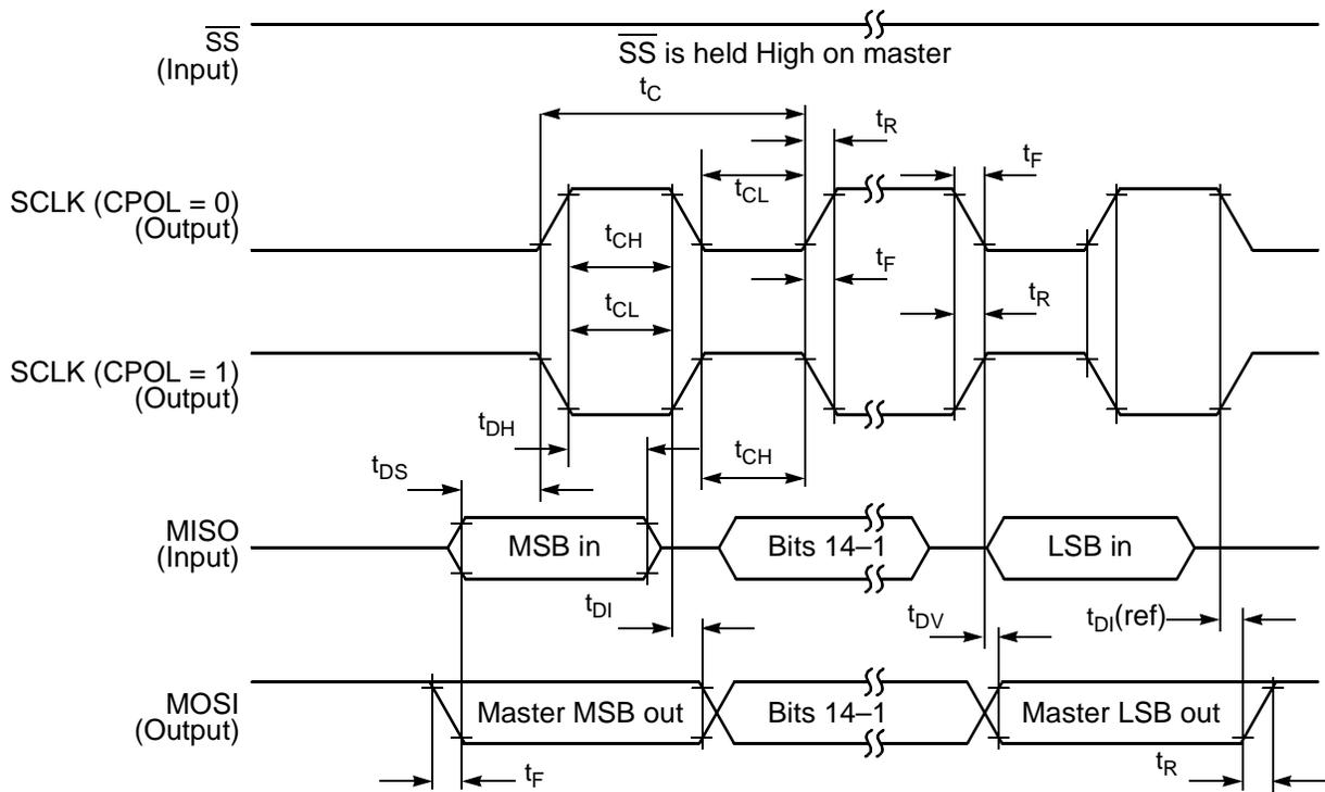
**Figure 22. SPI Master Timing (CPHA = 0)**
