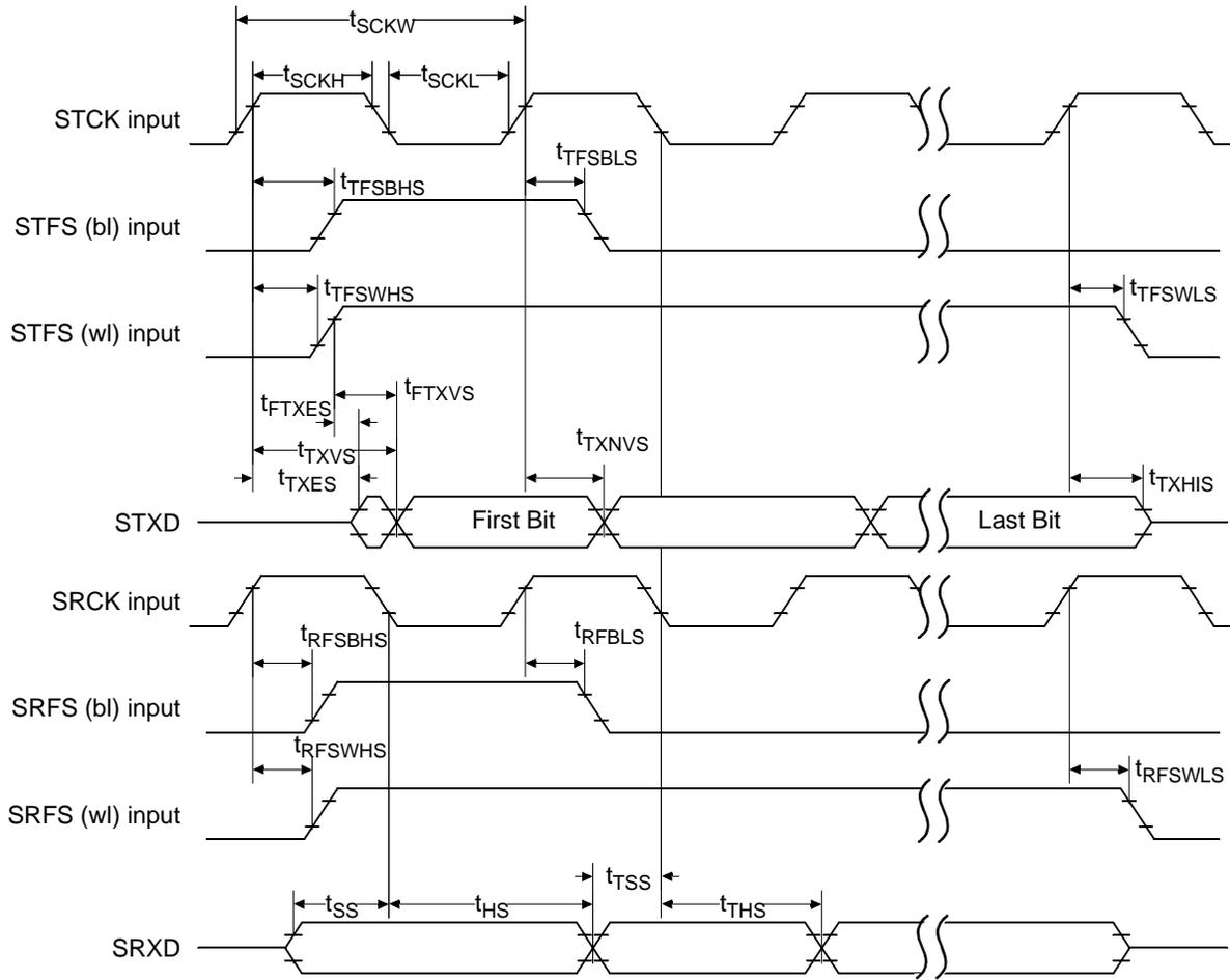
Figure 27. Slave Mode Clock Timing
