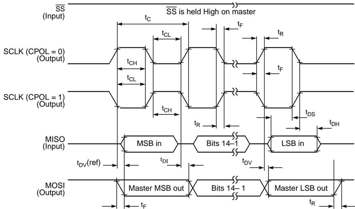
**Figure 23. SPI Master Timing (CPHA = 1)**
