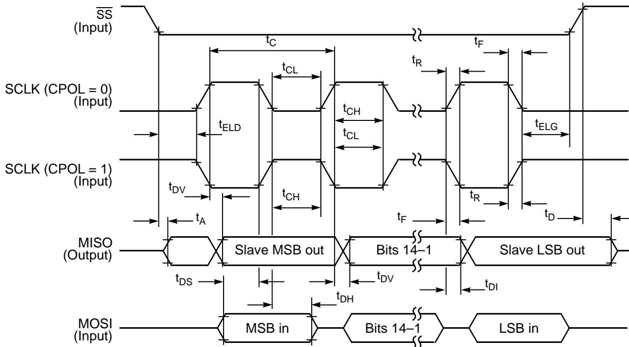
Figure 25. SPI Slave Timing (CPHA = 1)
