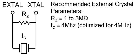
**Figure 11. Connecting to a Crystal Oscillator Circuit**
