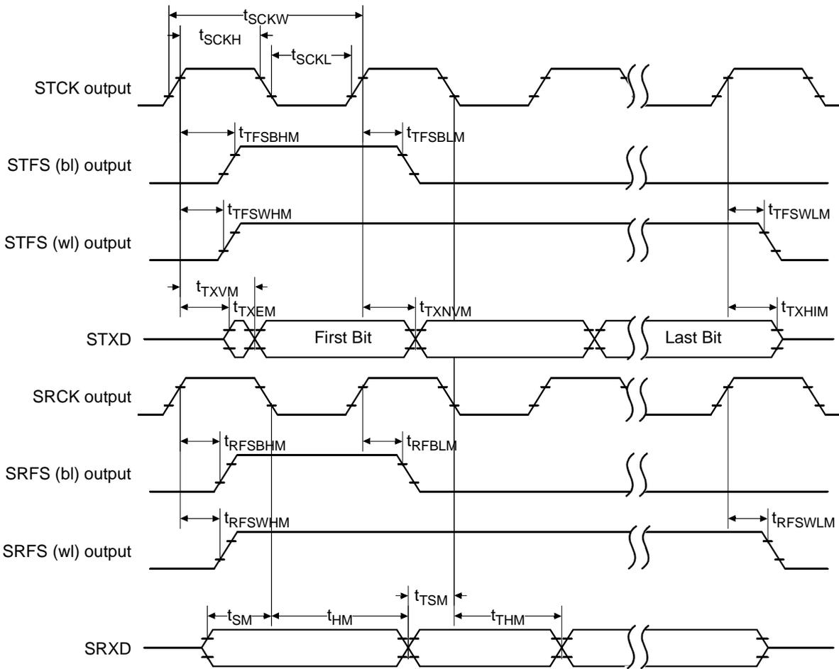
Figure 26. Master Mode Timing Diagram
