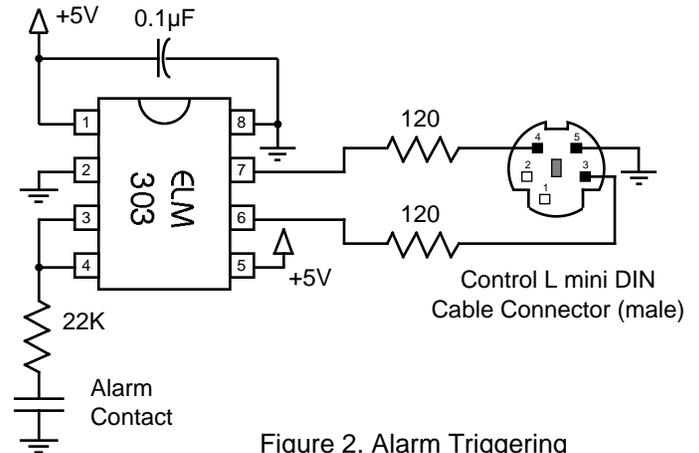
Figure 2. Alarm Triggering
