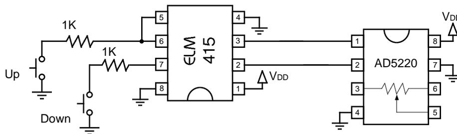
Figure 3. Controlling a digital potentiometer (with rapid down)
