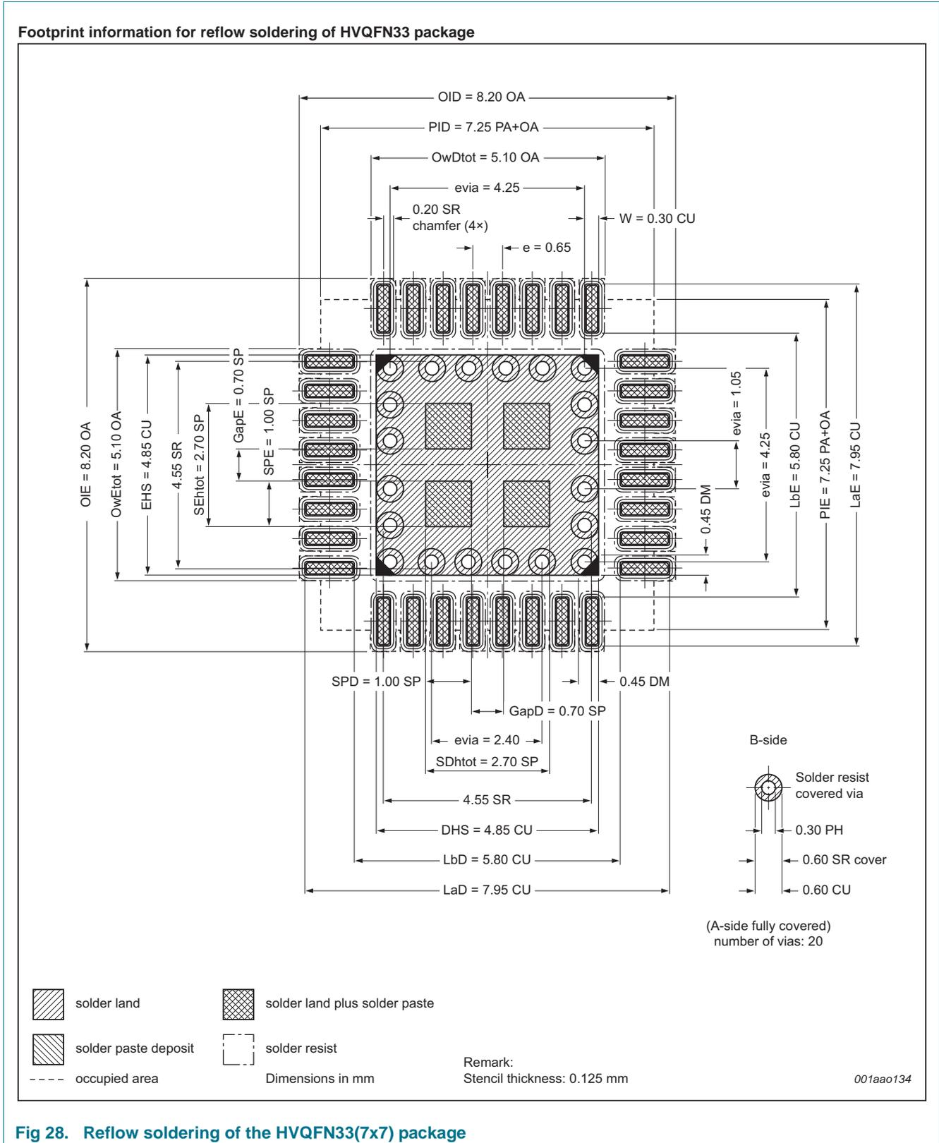
Fig 28. Reflow soldering of the HVQFN33(7x7) package
