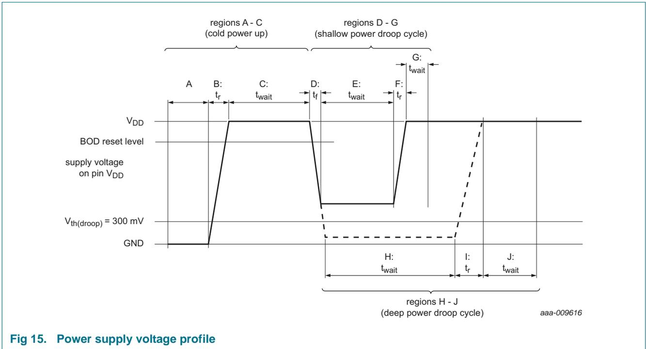
Fig 15. Power supply voltage profile
