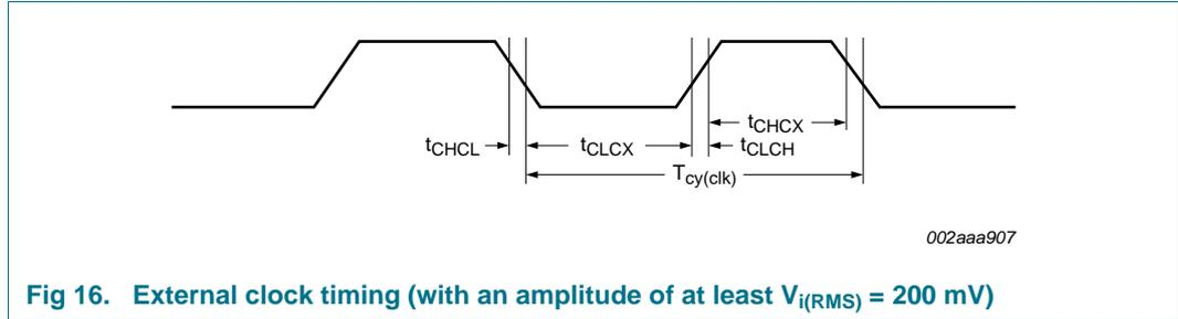
Fig 16. External clock timing (with an amplitude of at least  $V_{i(RMS)} = 200\text{ mV}$ )
