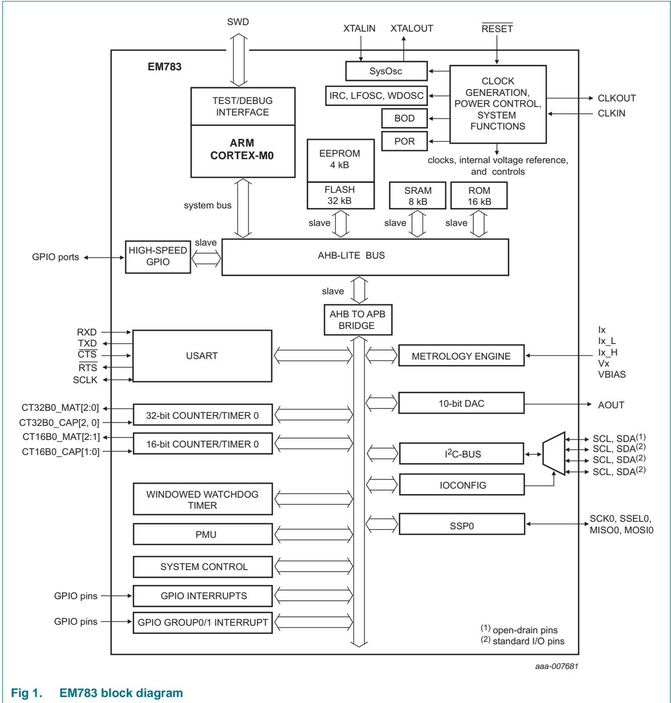
Fig 1. EM783 block diagram
