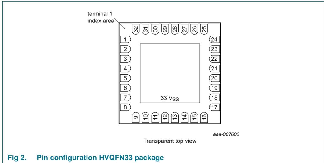
Fig 2. Pin configuration HVQFN33 package
