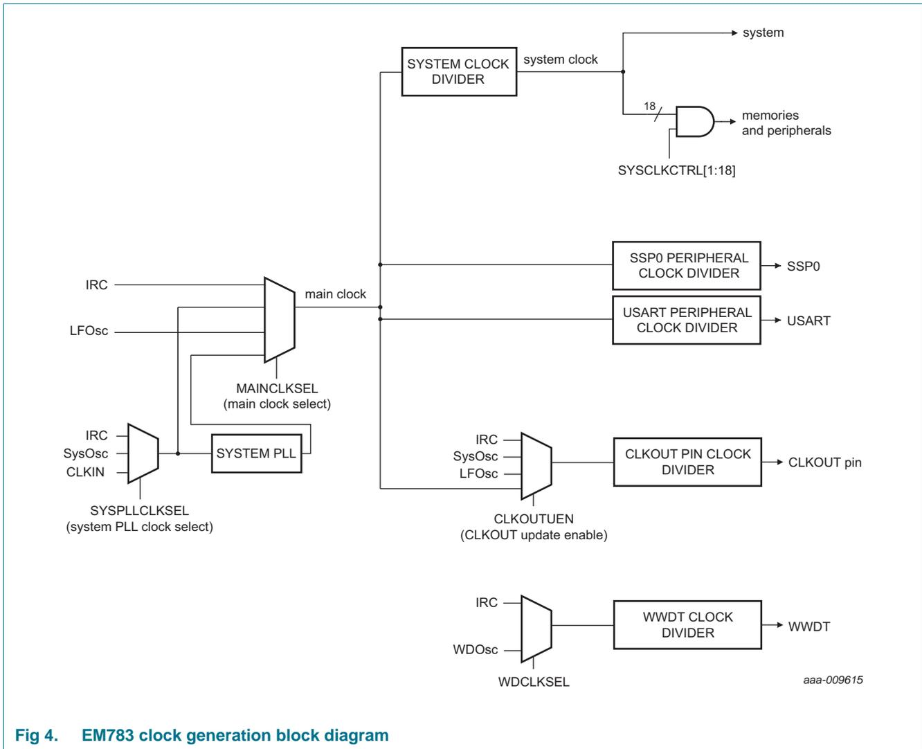
Fig 4. EM783 clock generation block diagram
