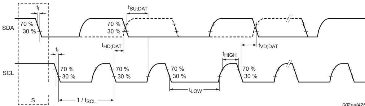
**Fig 18. I<sup>2</sup>C-bus pins clock timing**
