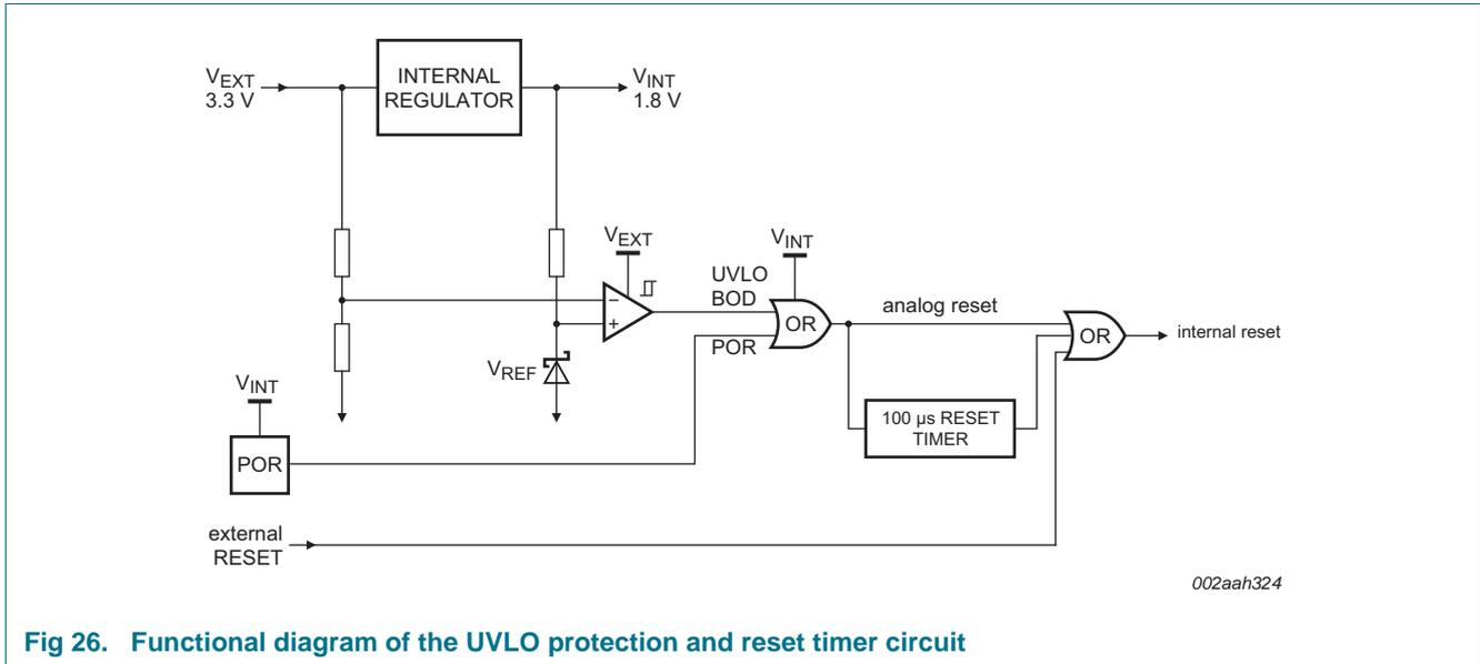
Fig 26. Functional diagram of the UVLO protection and reset timer circuit
