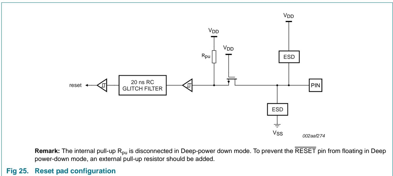
Fig 25. Reset pad configuration
