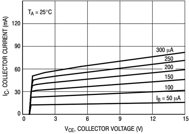
Figure 1.  $I_C - V_{CE}$
