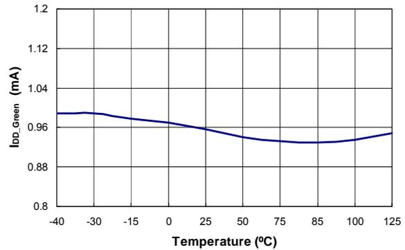
**Figure 11. Green-Mode Operating Supply Current (I<sub>DD-GREEN</sub>) vs. Temperature**
