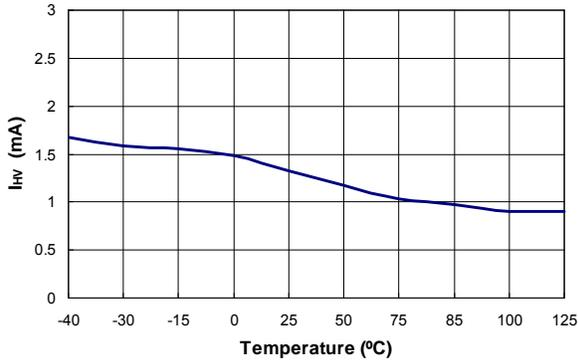
**Figure 14. Supply Current Drawn from Pin HV (I<sub>HV</sub>) vs. Temperature**
