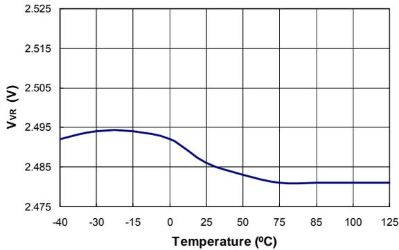
**Figure 10. Reference Voltage (V<sub>VR</sub>) vs. Temperature**
