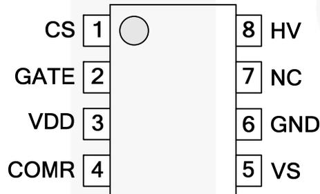
Figure 5. Pin Configuration
