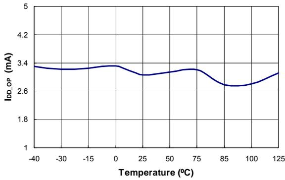
**Figure 8. Operating Current (I<sub>DD-OP</sub>) vs. Temperature**
