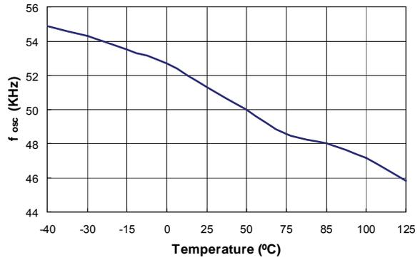
**Figure 9. Center Frequency (f<sub>OSC</sub>) vs. Temperature**
