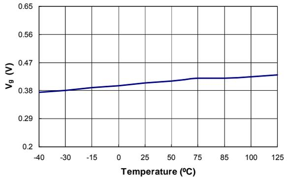
**Figure 17. Green Mode Ending Voltage on EA\_V (V<sub>G</sub>) vs. Temperature**
