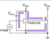
Figure 43. Current Path for MOSFET Turn-On
