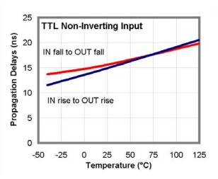
Figure 29. Propagation Delay vs. Temperature
