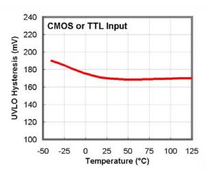
Figure 23. UVLO Hysteresis vs. Temperature
