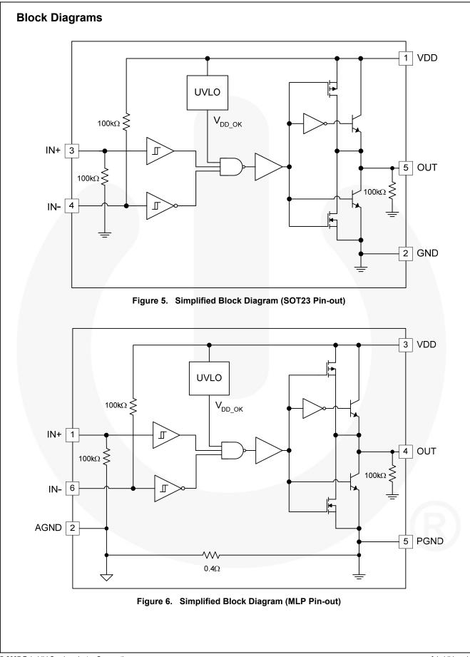
FAN3100 — Single 2A High-Speed, Low-Side Gate Driver
