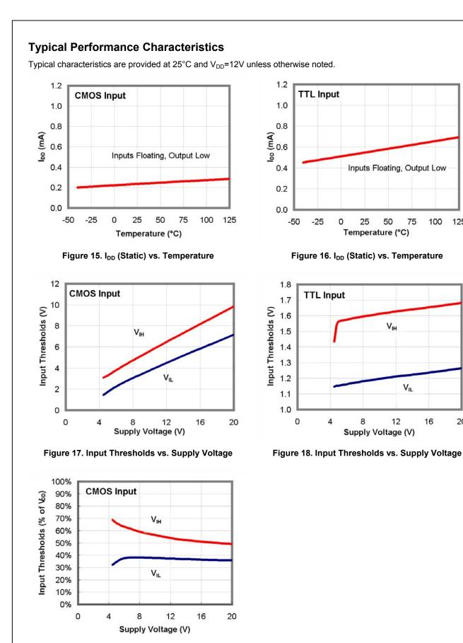
Typical characteristics are provided at 25°C and  $V_{DD}$ =12V unless otherwise noted.
