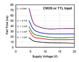
Figure 32. Fall Time vs. Supply Voltage
