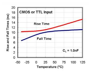
Figure 34. Rise and Fall Time vs. Temperature
