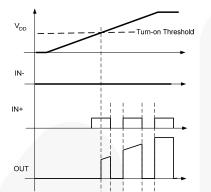
Figure 47. Non-Inverting Start-Up Waveforms
