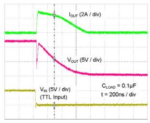
Figure 38. Quasi-Static Sink Current with  $V_{DD}$ =12V
