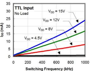
Figure 12. I<sub>DD</sub> (No-Load) vs. Frequency
