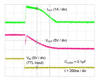
Figure 40. Quasi-Static Sink Current with V<sub>DD</sub>=8V
