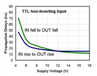
Figure 27. Propagation Delay vs. Supply Voltage
