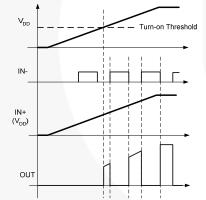
Figure 48. Inverting Start-Up Waveforms
