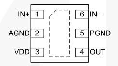
Figure 3. 2x2mm 6-Lead MLP (Top View)
