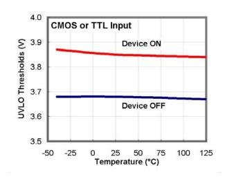
Figure 22. UVLO Thresholds vs. Temperature
