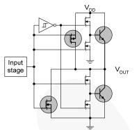
Figure 42. MillerDrive™ Output Architecture
