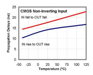
Figure 28. Propagation Delay vs. Temperature
