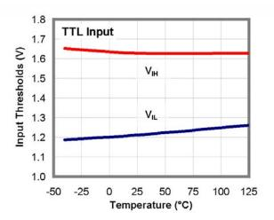
Figure 21. TTL Input Thresholds vs. Temperature
