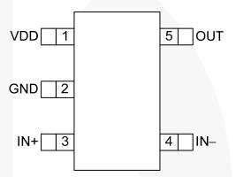
Figure 4. SOT23-5 (Top View)
