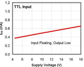
Figure 10. I<sub>DD</sub> (Static) vs. Supply Voltage
