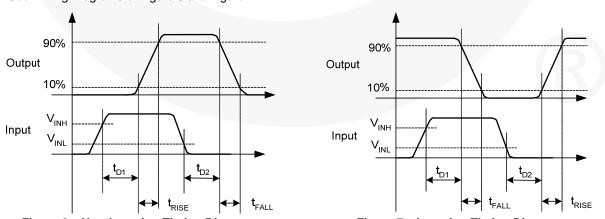
Figure 6. Non-Inverting Timing Diagram
