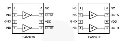
Figure 3. Pin Configurations (Repeated)
