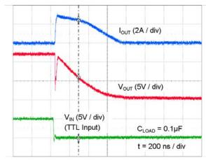
Figure 25. Quasi-Static Sink Current with  $V_{DD}$ =12 $V^{(11)}$
