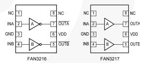
Figure 1. Pin Configurations
