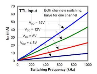
Figure 10. I<sub>DD</sub> (No-Load) vs. Frequency
