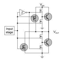
Figure 29. MillerDrive™ Output Architecture
