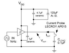
Figure 28. Quasi-Static I<sub>OUT</sub> / V<sub>OUT</sub> Test Circuit
