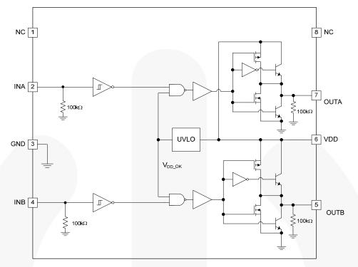
Figure 4. FAN3216 Block Diagram
