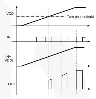
Figure 33. Inverting Startup Waveforms
