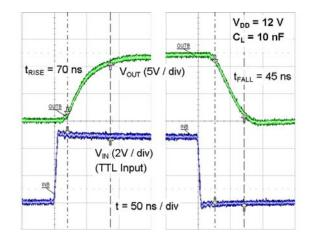
Figure 23. Rise/Fall Waveforms with 10nF Load
