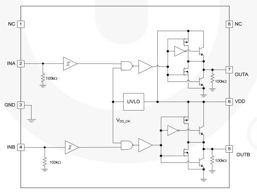
Figure 5. FAN3217 Block Diagram
