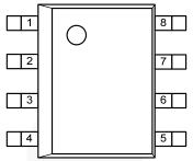
Figure 2. SOIC-8 (Top View)
