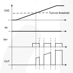
Figure 32. Non-Inverting Startup Waveforms
