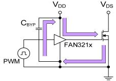
Figure 30. Current Path for MOSFET Turn-On
