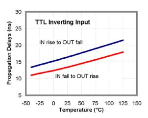
Figure 17. Propagation Delays vs. Temperature
