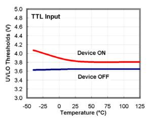
Figure 14. UVLO Threshold vs. Temperature
