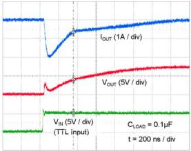
Figure 26. Quasi-Static Source Current with V<sub>DD</sub>=8V<sup>(11)</sup>
