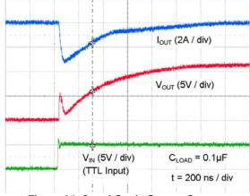
Figure 24. Quasi-Static Source Current with V<sub>DD</sub>=12V<sup>(11)</sup>
