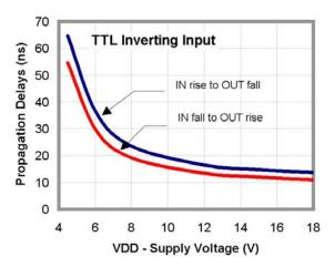
Figure 15. Propagation Delay vs. Supply Voltage
