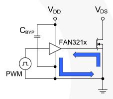
Figure 31. Current Path for MOSFET Turn-Off
