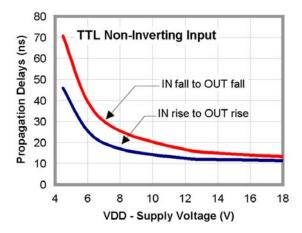
Figure 16. Propagation Delay vs. Supply Voltage
