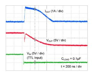
Figure 27. Quasi-Static Sink Current with V<sub>DD</sub>=8V<sup>(11)</sup>
