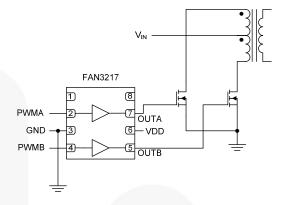
Figure 35. Primary-side Dual Driver in a Push-pull Converter
