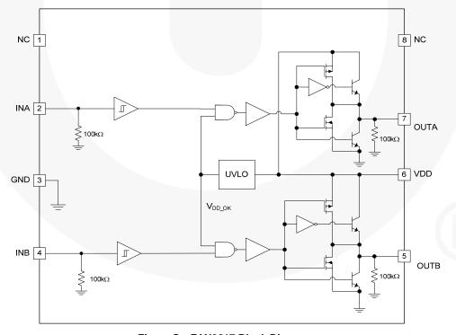
Figure 5. FAN3217 Block Diagram
