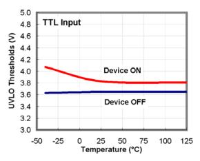
Figure 14. UVLO Threshold vs. Temperature
