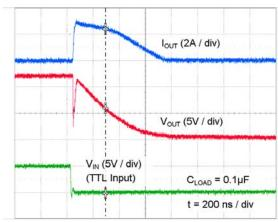
Figure 25. Quasi-Static Sink Current with V<sub>DD</sub>=12V<sup>(11)</sup>
