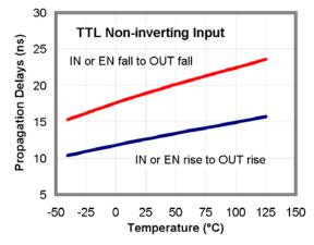
Figure 18. Propagation Delays vs. Temperature
