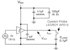
Figure 28. Quasi-Static I<sub>OUT</sub> / V<sub>OUT</sub> Test Circuit
