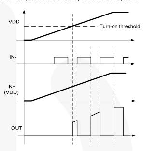
Figure 33. Inverting Startup Waveforms
