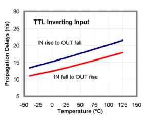
Figure 17. Propagation Delays vs. Temperature
