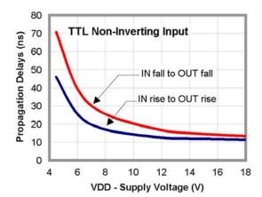
Figure 16. Propagation Delay vs. Supply Voltage
