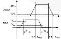
Figure 6. Non-Inverting Timing Diagram
