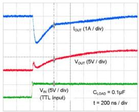
Figure 26. Quasi-Static Source Current with V<sub>DD</sub>=8V<sup>(11)</sup>
