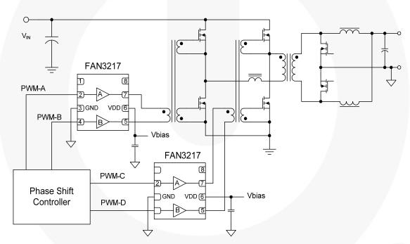
Figure 36. Phase-shifted Full-bridge with Two Gate Drive Transformers (Simplified)
