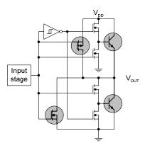
Figure 29. MillerDrive™ Output Architecture
