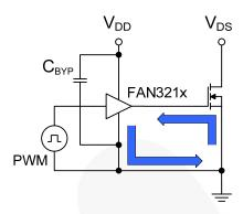
Figure 31. Current Path for MOSFET Turn-Off
