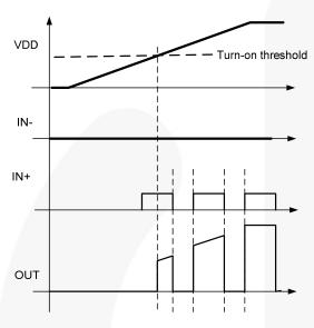
Figure 32. Non-Inverting Startup Waveforms
