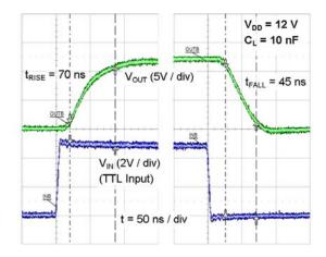
Figure 23. Rise/Fall Waveforms with 10nF Load
