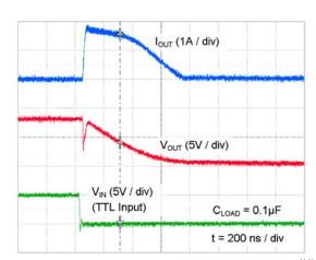
Figure 27. Quasi-Static Sink Current with V<sub>DD</sub>=8V<sup>(11)</sup>
