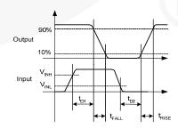
Figure 7. Inverting Timing Diagram
