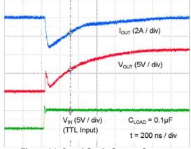
Figure 24. Quasi-Static Source Current with V<sub>DD</sub>=12V<sup>(11)</sup>
