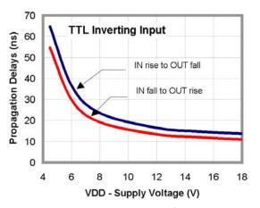
Figure 15. Propagation Delay vs. Supply Voltage
