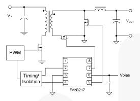
Figure 34. Forward Converter with Synchronous Rectification
