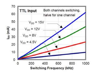
Figure 10. I<sub>DD</sub> (No-Load) vs. Frequency
