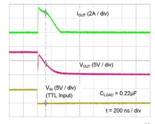
Figure 43. Quasi-Static Sink Current with V<sub>DD</sub>=12V<sup>(14)</sup>
