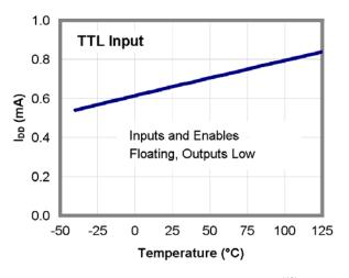
Figure 19. I<sub>DD</sub> (Static) vs. Temperature<sup>(13)</sup>
