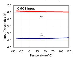
Figure 25. Input Thresholds vs. Temperature
