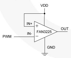
Figure 51. Dual-Input Driver Enabled, Inverting Configuration
