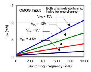
Figure 15. IDD (No-Load) vs. Frequency
