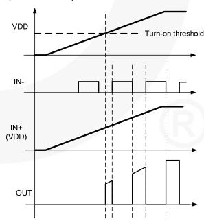
Figure 53. Inverting Startup Waveforms
