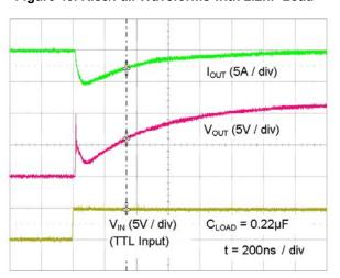
Figure 42. Quasi-Static Source Current with  $V_{DD}$ =12 $V^{(14)}$
