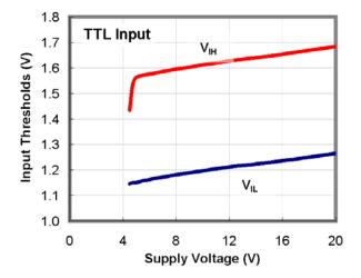
Figure 22. Input Thresholds vs. Supply Voltage
