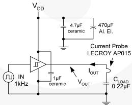
Figure 46. Quasi-Static I<sub>OUT</sub> / V<sub>OUT</sub> Test Circuit
