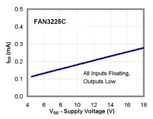
Figure 14. I<sub>DD</sub> (Static) vs. Supply Voltage<sup>(13)</sup>
