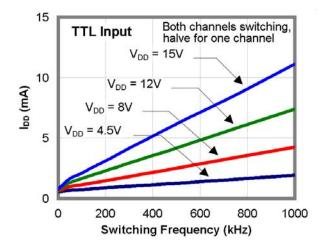
Figure 16. I<sub>DD</sub> (No-Load) vs. Frequency
