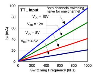
Figure 17. I<sub>DD</sub> (2.2nF Load) vs. Frequency
