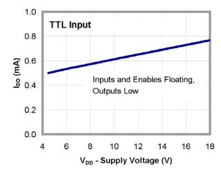
Figure 12. I<sub>DD</sub> (Static) vs. Supply Voltage<sup>(13)</sup>
