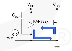
Figure 49. Current Path for MOSFET Turn-off
