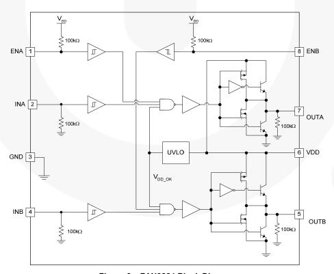
Figure 6. FAN3224 Block Diagram
