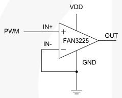
Figure 50. Dual-Input Driver Enabled, Non-Inverting Configuration
