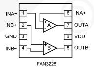
Figure 1. Pin Configurations
