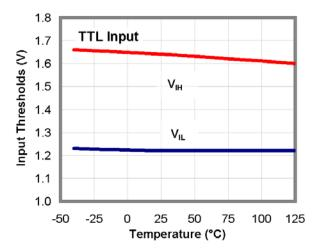
Figure 26. Input Thresholds vs. Temperature
