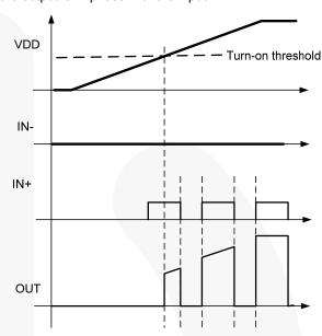
Figure 52. Non-Inverting Start-Up Waveforms
