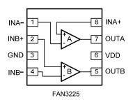
Figure 4. Pin Assignments (Repeated)
