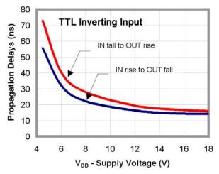
Figure 29. Propagation Delay vs. Supply Voltage
