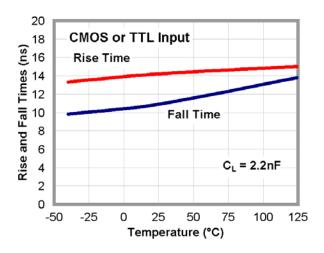
Figure 39. Rise and Fall Times vs. Temperature
