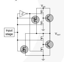
Figure 47. MillerDrive™ Output Architecture
