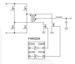
Figure 54. High Current Forward Converter with Synchronous Rectification
