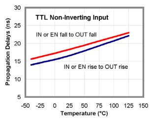
Figure 35. Propagation Delays vs. Temperature
