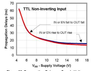
Figure 31. Propagation Delay vs. Supply Voltage
