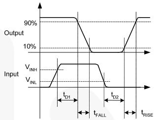
Figure 8. Non-Inverting (EN HIGH or Floating)
