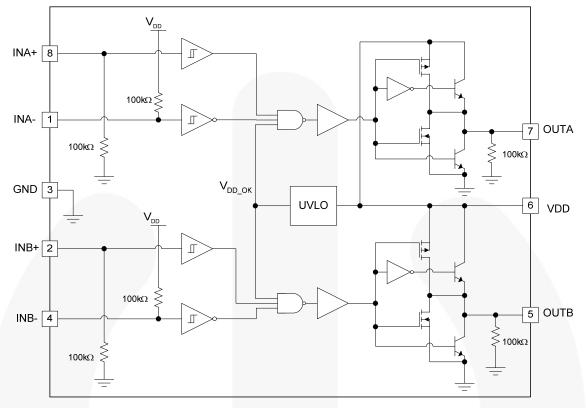
Figure 7. FAN3225 Block Diagram
