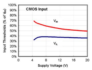
Figure 24. Input Threshold % vs. Supply Voltage
