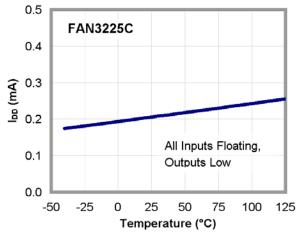
Figure 21. I<sub>DD</sub> (Static) vs. Temperature<sup>(13)</sup>
