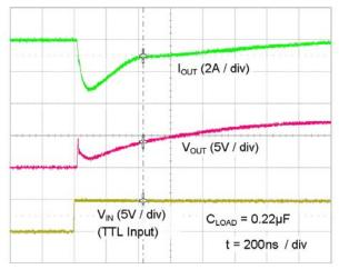
$I_{OUT}$  (2A / div)  $V_{OUT}$  (5V / div)  $V_{IN}$  (5V / div)  $C_{LOAD} = 0.22 \mu F$  t = 200 ns / div
