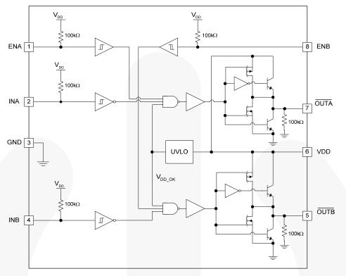
Figure 5. FAN3223 Block Diagram
