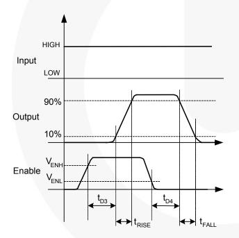
Figure 10. Non-Inverting (IN HIGH)
