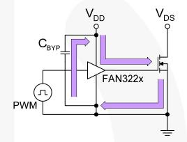
Figure 48. Current Path for MOSFET Turn-on
