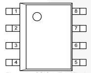
Figure 3. SOIC-8 (Top View)
