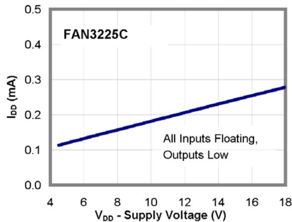
Figure 14.  $I_{DD}$  (Static) vs. Supply Voltage<sup>(13)</sup>
