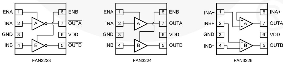
Figure 1. Pin Configurations
