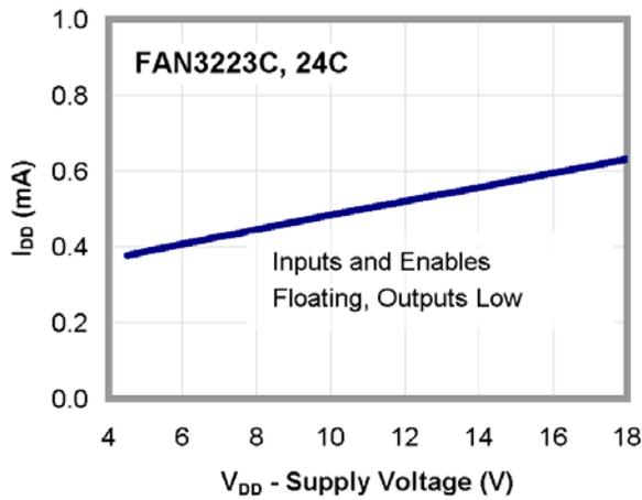
Figure 12.  $I_{DD}$  (Static) vs. Supply Voltage<sup>(13)</sup>
