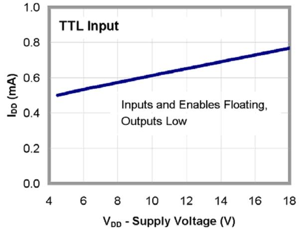
Figure 13.  $I_{DD}$  (Static) vs. Supply Voltage<sup>(13)</sup>
