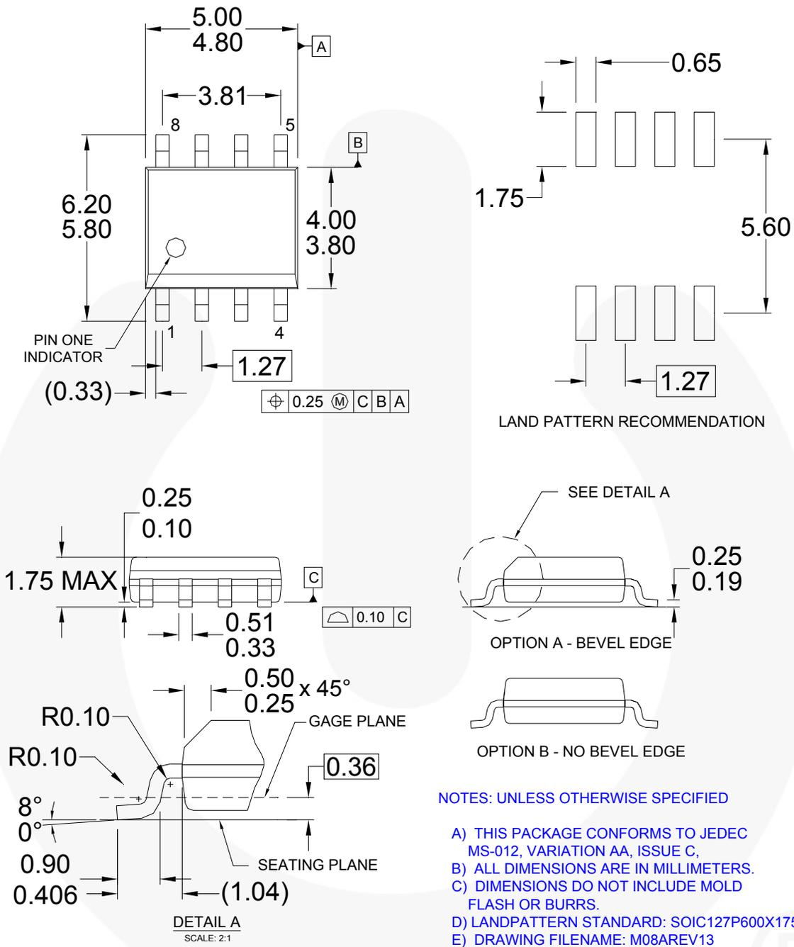
Figure 58. 8-Lead SOIC
