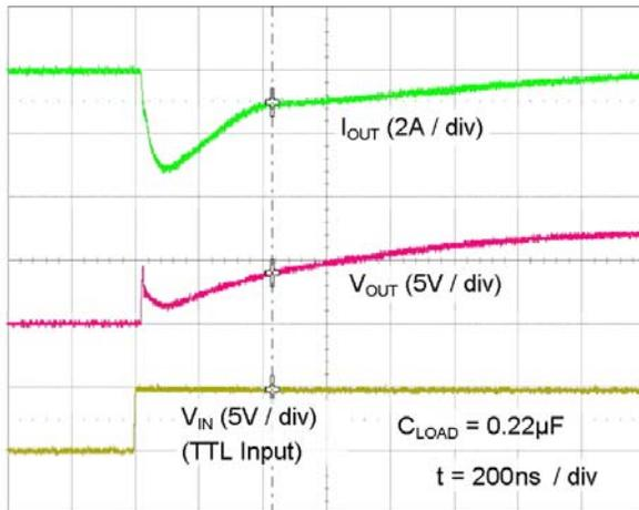
Figure 44. Quasi-Static Source Current with  $V_{DD}=8V^{(14)}$
