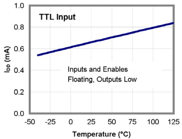
Figure 20.  $I_{DD}$  (Static) vs. Temperature<sup>(13)</sup>
