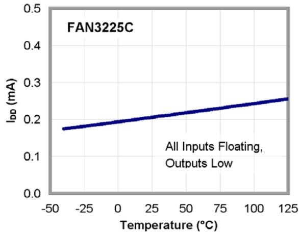
Figure 21.  $I_{DD}$  (Static) vs. Temperature<sup>(13)</sup>
