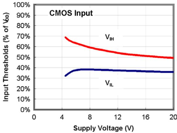
Figure 24. Input Threshold % vs. Supply Voltage
