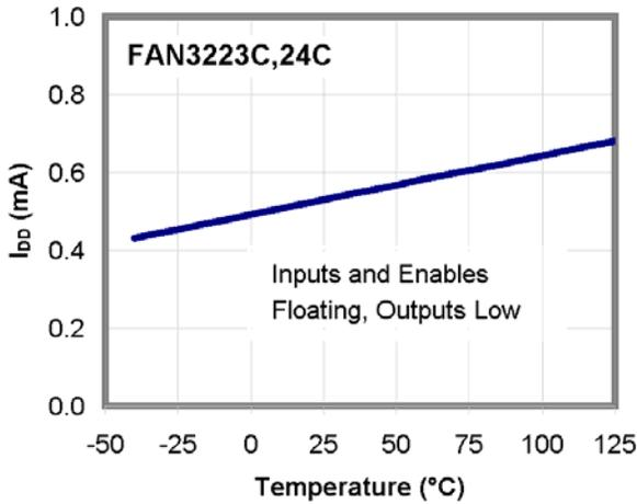
Figure 19.  $I_{DD}$  (Static) vs. Temperature<sup>(13)</sup>
