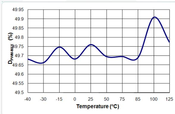
Figure 22. D<sub>PWM-MAX</sub> vs. Temperature
