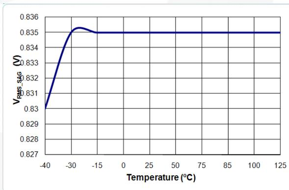
Figure 24. V<sub>RMS-SAG</sub> vs. Temperature
