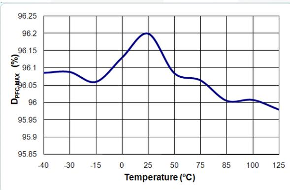
Figure 21. D<sub>PFC-MAX</sub> vs. Temperature
