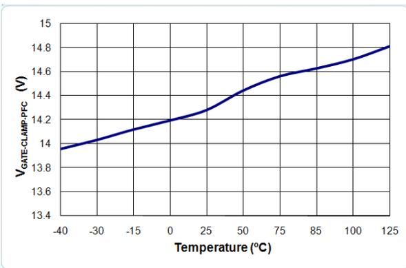
Figure 19. V<sub>GATE-CLAMP-PFC</sub> vs. Temperature
