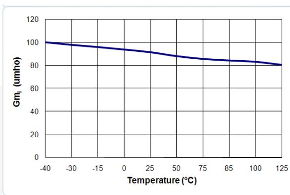
Figure 14. Gm<sub>I</sub> vs. Temperature
