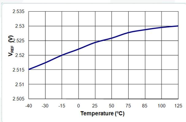
Figure 12. V<sub>REF</sub> vs. Temperature
