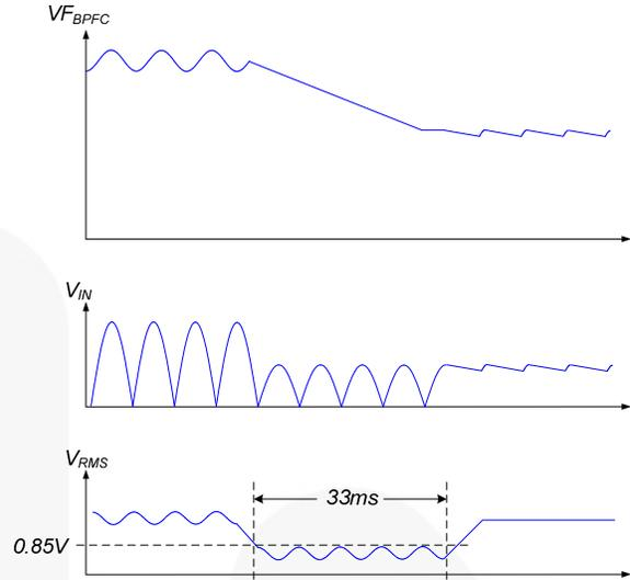
Figure 37. The First Condition of Sag Protection
