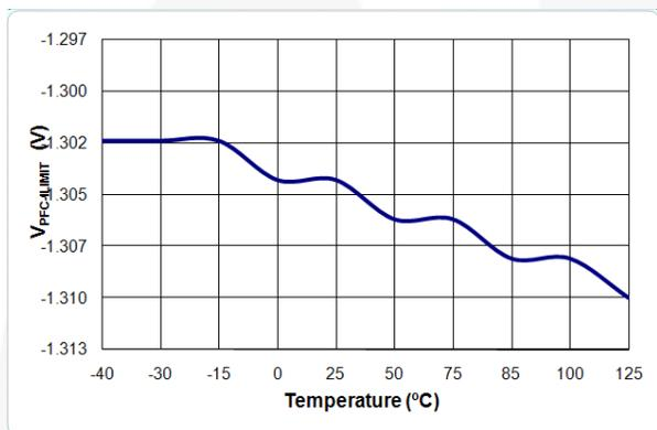
Figure 15. V<sub>PFC-ILIMIT</sub> vs. Temperature
