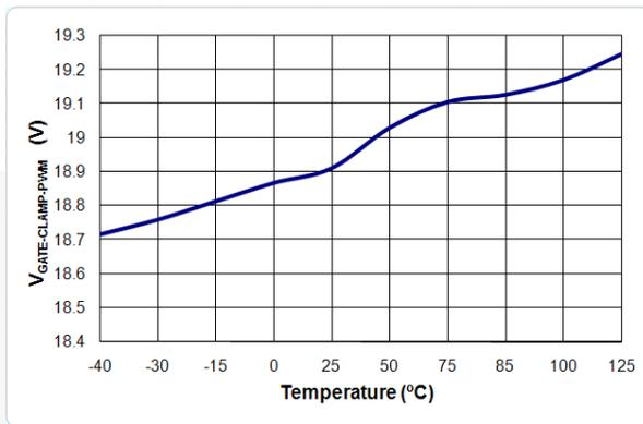
Figure 20. V<sub>GATE-CLAMP-PWM</sub> vs. Temperature
