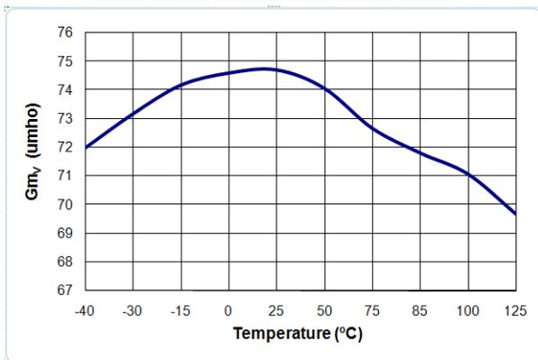
Figure 13. Gm<sub>V</sub> vs. Temperature
