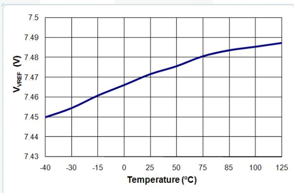
Figure 10. V<sub>VREF</sub> vs. Temperature
