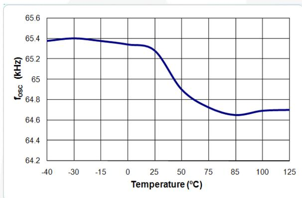
Figure 9. f<sub>osc</sub> vs. Temperature
