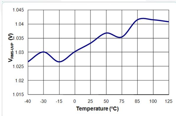
Figure 17. V<sub>RMS-UVP</sub> vs. Temperature
