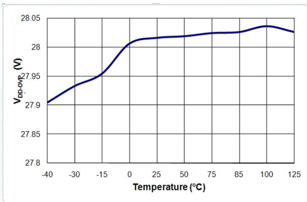
Figure 8. V<sub>DD-OVP</sub> vs. Temperature
