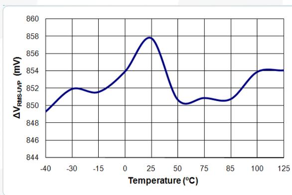
Figure 18. ΔV<sub>RMS-UVP</sub> vs. Temperature
