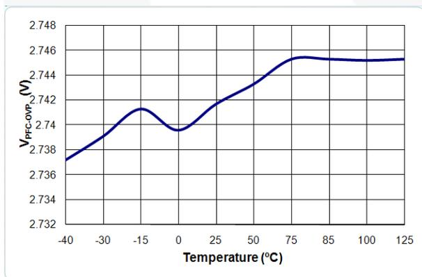
Figure 11. V<sub>PFC-OVP</sub> vs. Temperature
