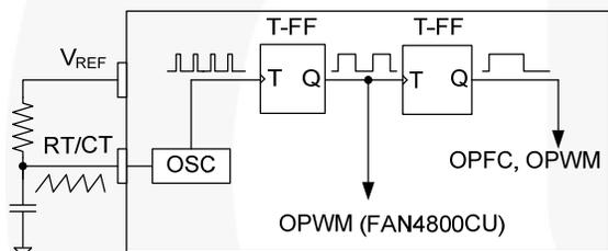
Figure 25. Oscillator Configuration
