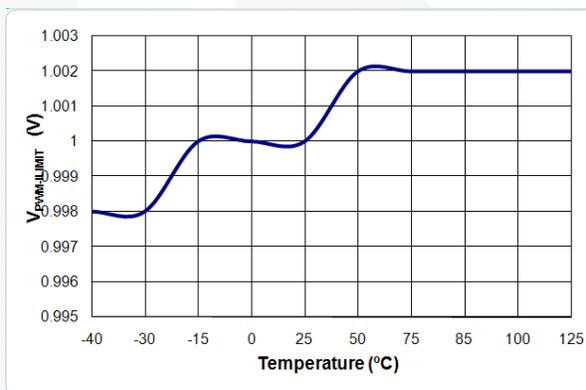
Figure 16. V<sub>PWM-ILIMIT</sub> vs. Temperature
