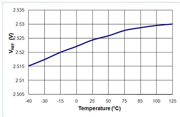
Figure 12. V<sub>REF</sub> vs. Temperature
