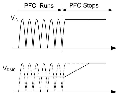
**Figure 31.  $V_{RMS}$  According to the PFC Operation**
