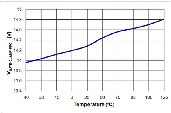
Figure 19. V<sub>GATE-CLAMP-PFC</sub> vs. Temperature
