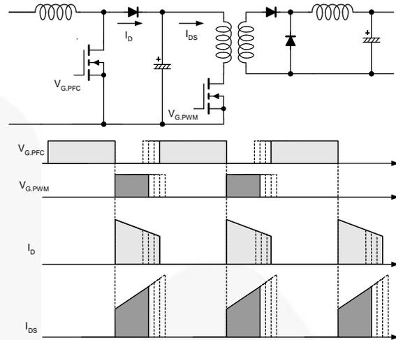
Figure 27. Interleaved Leading / Trailing Edge Modulation
