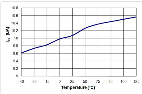
Figure 23. I<sub>SS</sub> vs. Temperature
