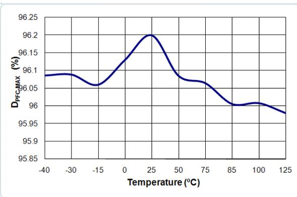
Figure 21. D<sub>PFC-MAX</sub> vs. Temperature
