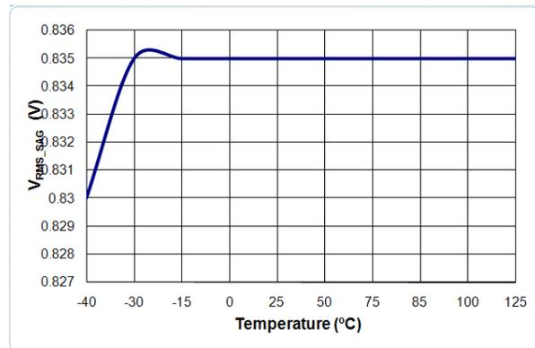
Figure 24. V<sub>RMS-SAG</sub> vs. Temperature
