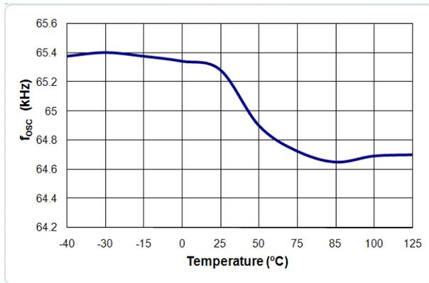
Figure 9. f<sub>osc</sub> vs. Temperature
