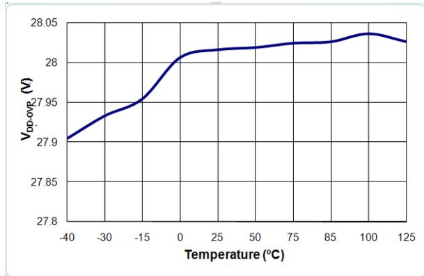
Figure 8. V<sub>DD-OVP</sub> vs. Temperature
