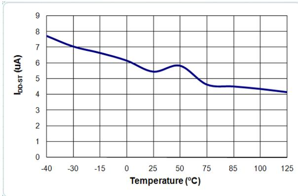
Figure 7. I<sub>DD-ST</sub> vs. Temperature
