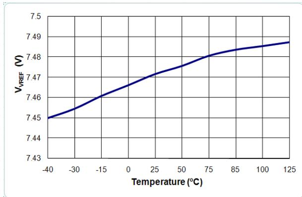
Figure 10. V<sub>VREF</sub> vs. Temperature
