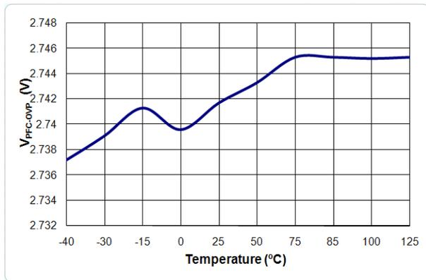
Figure 11. V<sub>PFC-OVP</sub> vs. Temperature
