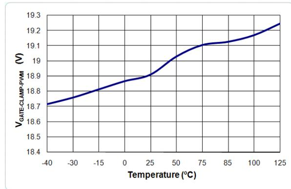
Figure 20. V<sub>GATE-CLAMP-PWM</sub> vs. Temperature
