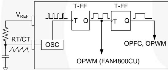
Figure 25. Oscillator Configuration
