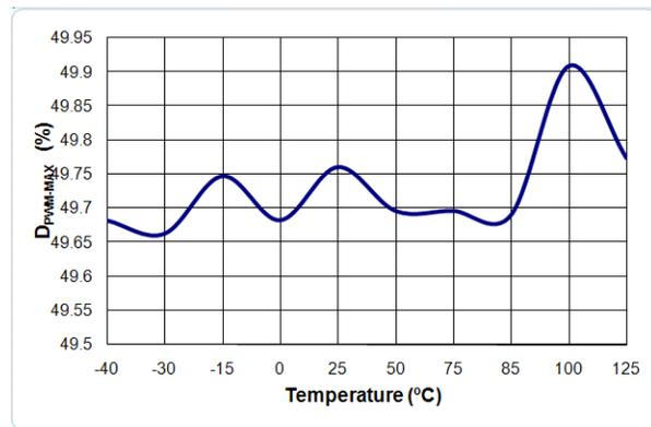
Figure 22. D<sub>PWM-MAX</sub> vs. Temperature
