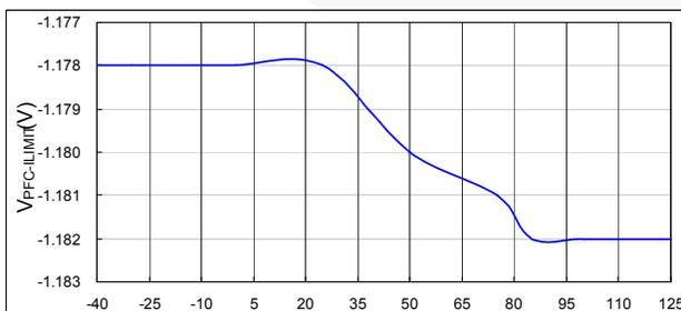
Figure 16. V<sub>PFC-ILIMIT</sub> vs. Temperature
