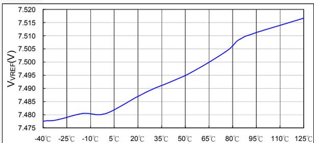
Figure 11. V<sub>VREF</sub> vs. Temperature
