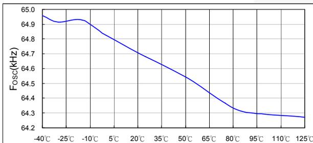
Figure 10. f<sub>osc</sub> vs. Temperature
