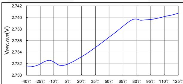
Figure 12. V<sub>PFC-OVP</sub> vs. Temperature
