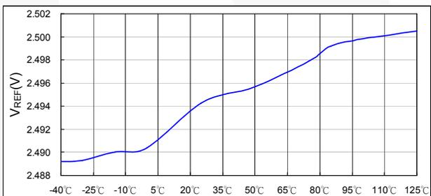
Figure 13. V<sub>REF</sub> vs. Temperature
