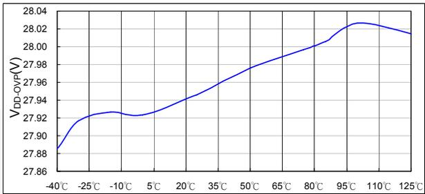
Figure 9. V<sub>DD-OVP</sub> vs. Temperature
