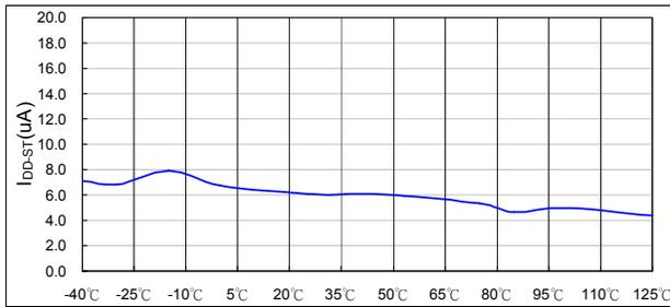
Figure 8. I<sub>DD-ST</sub> vs. Temperature
