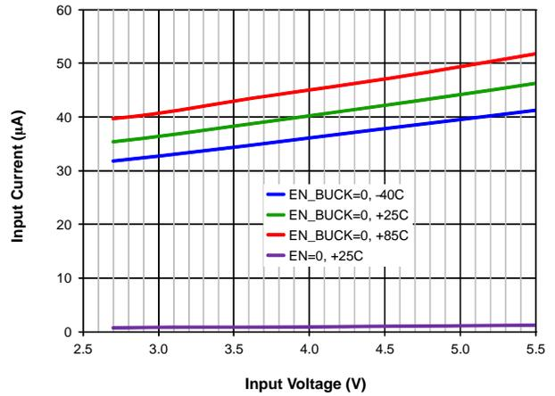
Figure 10. Shutdown Current vs. Input Voltage, Over-Temperature
