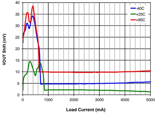
**Figure 5. Output Regulation vs. Load Current, Over-Temperature**
