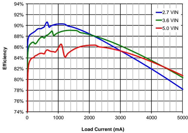
**Figure 3. Efficiency vs. Load Current and Input Voltage**
