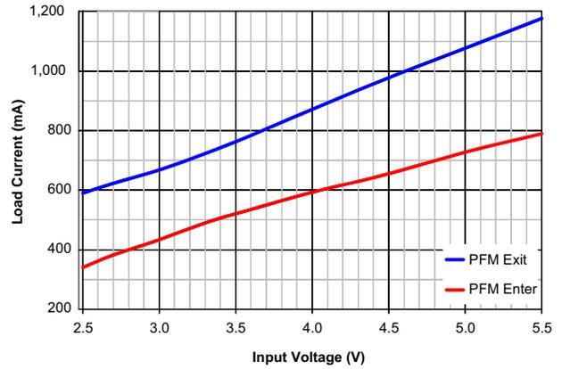
**Figure 6. PFM Entry / Exit Level vs. Input Voltage**
