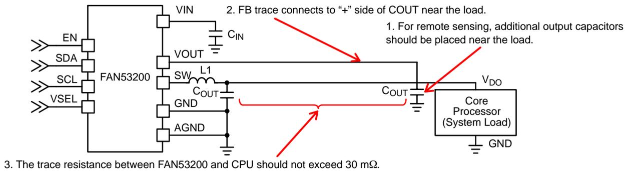
3. The trace resistance between FAN53200 and CPU should not exceed 30 mΩ.
