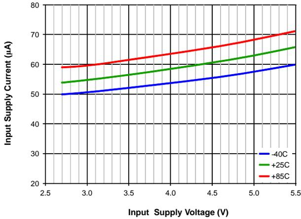
Figure 9. Quiescent Current vs. Input Voltage, Over-Temperature
