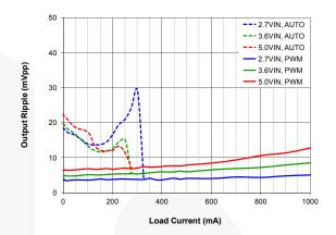
Figure 22. Output Ripple vs. Load Current and Input Voltage, V<sub>OUT</sub>=2.9 V, FPWM, Dotted for Auto Mode
