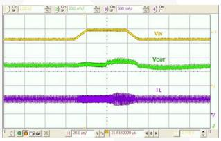
Figure 30. Line Transient, 3.3-3.9-3.3  $V_{\text{IN}},$  10  $\mu s$  Edge,  $V_{\text{OUT}}\text{=}2.9~V,\,58~\text{mA}$  Load
