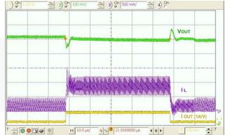
Figure 26. Load Transient,  $V_{IN}$ =5 V,  $V_{OUT}$ =3.3 V, 10-200-10 mA, 100 ns Edge
