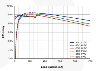
Figure 6. Efficiency vs. Load Current and Input Voltage, V<sub>OUT</sub>=2.9 V, Dotted for Decreasing Load
