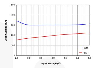
Figure 16. PFM / PWM Boundary vs. Input Voltage,
