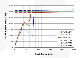
Figure 24. . Frequency vs. Load Current and Input Voltage,  $V_{\text{OUT}}$ =2.9 V, Auto Mode, Dotted for FPWM
