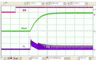
Figure 32. Combined Line / Load Transient,  $V_{\text{OUT}}$ =2.9V, 3.9-3.3-3.9  $V_{\text{IN}}$ , 10 µs Edge, 58-500-58 mA Load, 100 ns Edge
