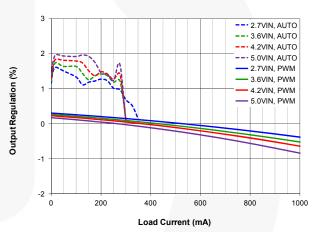
Figure 12.  $\Delta V_{OUT}$  (%) vs. Load Current and Input Voltage,  $V_{OUT}$ =1.82 V, Normalized to 3.6  $V_{IN}$ , 500mA Load, FPWM, Dotted for Auto Mode
