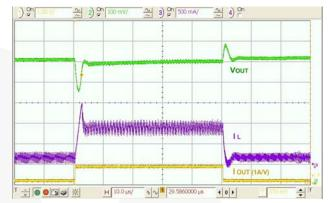
Figure 28. Load Transient, V<sub>IN</sub>=5 V, V<sub>OUT</sub>=2.9 V, 10-200-10 mA, 100 ns Edge
