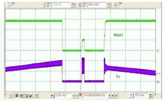
Figure 34. Startup, 4.7 Ω Load
