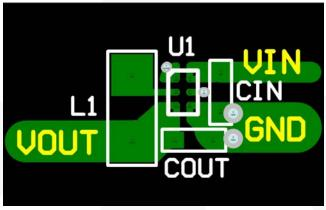
Figure 37. 3 MHz PCB Layout Guidance
