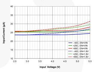
Figure 18. Quiescent Current vs. Input Voltage and Temperature, V<sub>OUT</sub>=2.9 V, EN=V<sub>IN</sub> Solid, Dotted for **EN=1.8 V**
