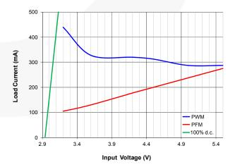
Figure 14. PFM / PWM /100% Duty Cycle Boundary vs. Input Voltage, V<sub>OUT</sub>=3.3 V
