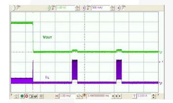
Figure 36. 250 mΩ Fault, Rapid Fault, FAN53600
