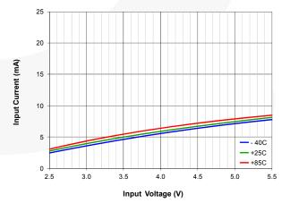
Figure 20. Quiescent Current vs. Input Voltage and Temperature, V<sub>OUT</sub>=2.9 V, Mode=EN=V<sub>IN</sub> (FPWM)
