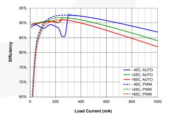
Figure 8. Efficiency vs. Load Current and Input Voltage, V<sub>OUT</sub>=1.82 V, Dotted for Decreasing Load
