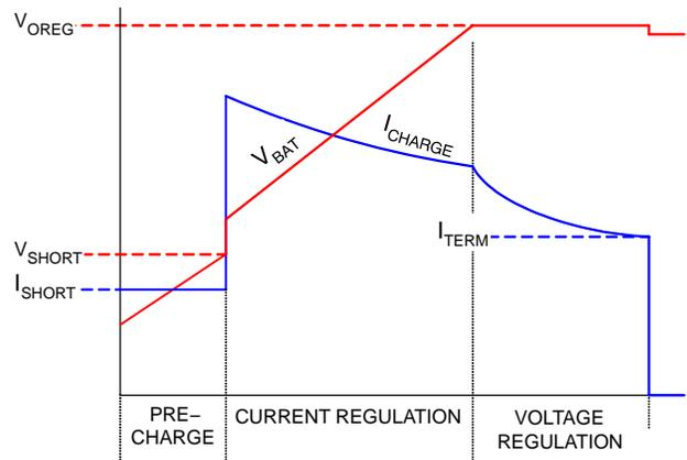
Figure 35. Charge Curve, I<sub>INLIM</sub> Limits I<sub>OCHARGE</sub>
