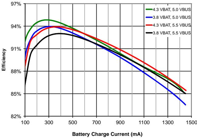
Figure 8. Charger Efficiency, No  $I_{INLIM}$ ,  $I_{OCHARGE}=1450\text{ mA}$
