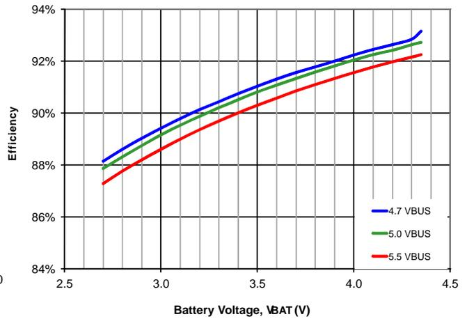
Figure 9. Charger Efficiency vs.  $V_{BUS}$ ,  $I_{INLIM}=500\text{ mA}$ ,  $V_{OREG}=4.35$
