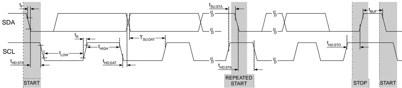
Figure 4. I<sup>2</sup>C Interface Timing for Fast and Slow Modes
