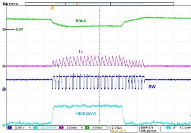
Figure 32. Load Transient, 5–155–5 mA,  $t_R=t_F=100\text{ ns}$
