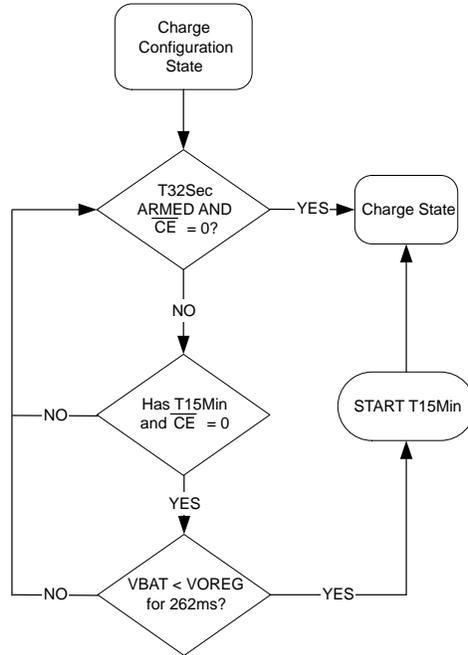
Figure 38. Charge Configuration
