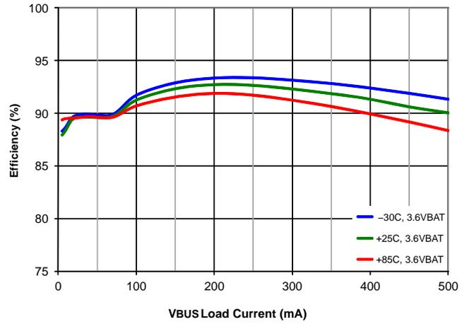
Figure 22. Efficiency Over-Temperature
