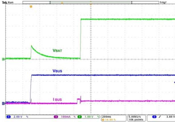
**Figure 18. No Battery, TE=0,  $V_{BUS}$  Power Up**
