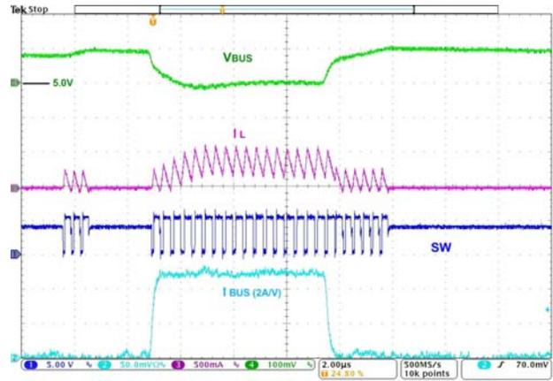
Figure 33. Load Transient, 5–255–5 mA,  $t_R=t_F=100\text{ ns}$
