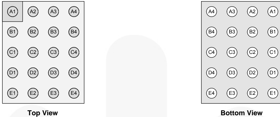
Figure 3. WLCSP-20 Pin Assignments
