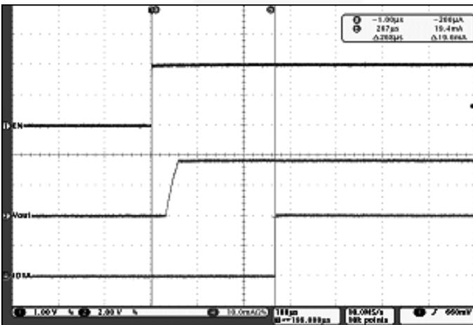
**Figure 15. Soft-Start with EN,  $V_{IN}=3.6V$ ,  $I_{LEDx}=20mA$**
