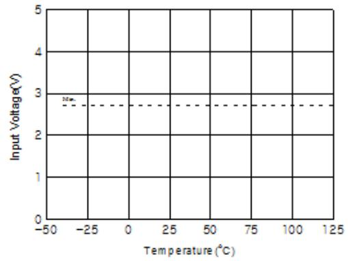
Figure 32. Logic High Input Voltage vs. Temperature
