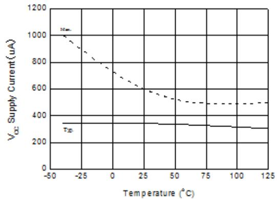
Figure 44.  $V_{CC}$  Supply Current vs. Temperature ( $V_{CC}=15\text{ V}$ )
