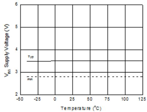
Figure 50.  $V_{BS}$  Under-Voltage Threshold (-) vs. Temperature
