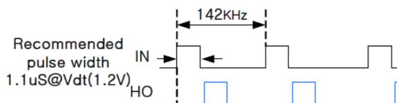
Figure 7. Recommendation of Pulse width Output Waveform
