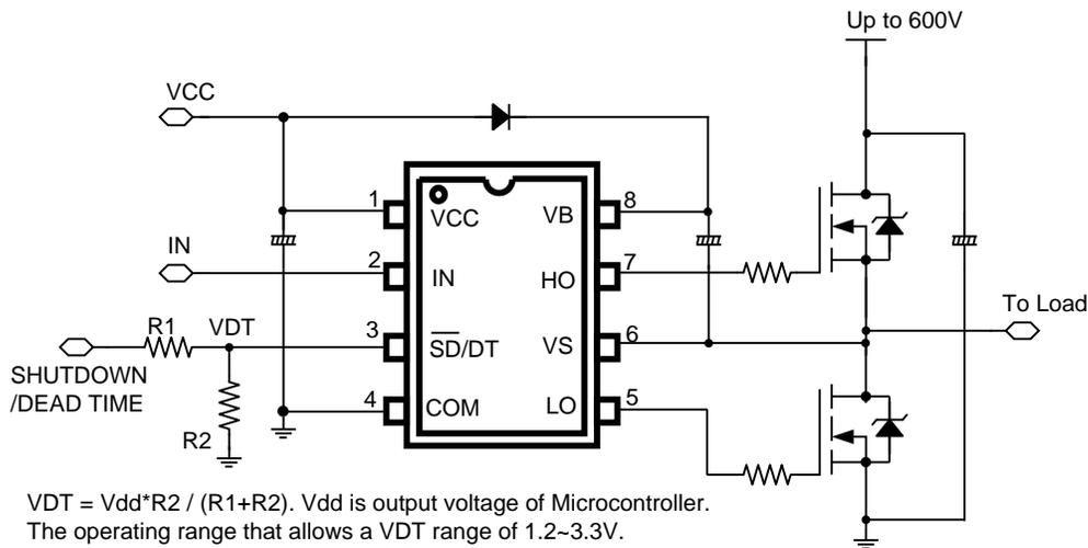
$VDT = V_{dd} * R2 / (R1 + R2)$ .  $V_{dd}$  is output voltage of Microcontroller.
