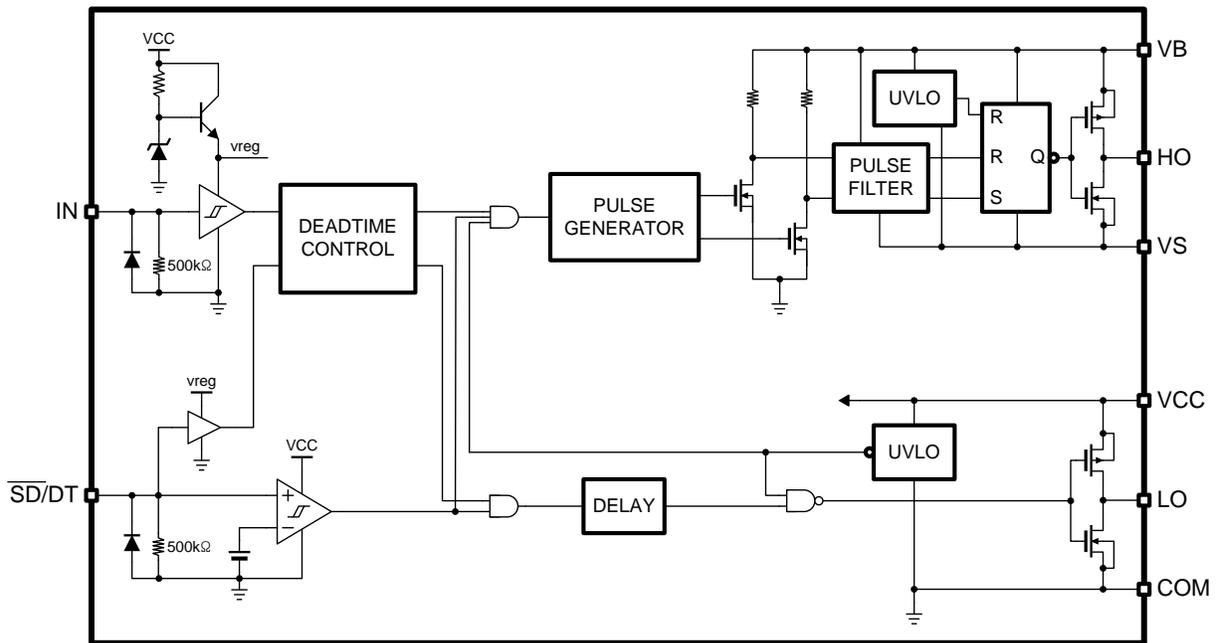
Figure 3. Block Diagram
