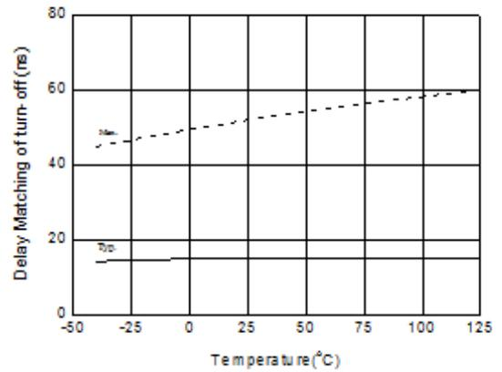
**Figure 60. Turn-off Delay Matching vs. Temperature**
