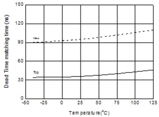
**Figure 58. Deadtime Matching Time vs. Temperature**
