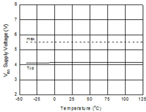
Figure 49.  $V_{BS}$  Under-Voltage Threshold (+) vs. Temperature
