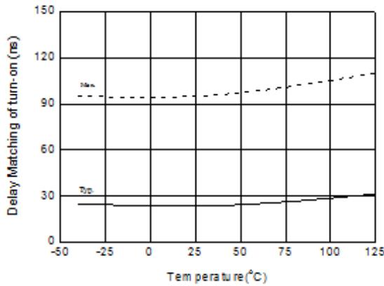
**Figure 59. Turn-on Delay Matching vs. Temperature**
