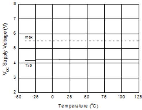
Figure 47.  $V_{CC}$  Under-Voltage Threshold (+) vs. Temperature
