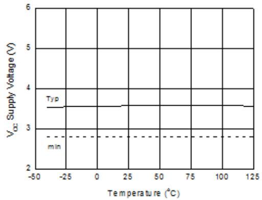
Figure 48.  $V_{CC}$  Under-Voltage Threshold (-) vs. Temperature
