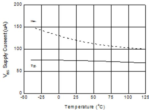
Figure 43.  $V_{BS}$  Supply Current vs. Temperature ( $V_{BS}=15\text{ V}$ )
