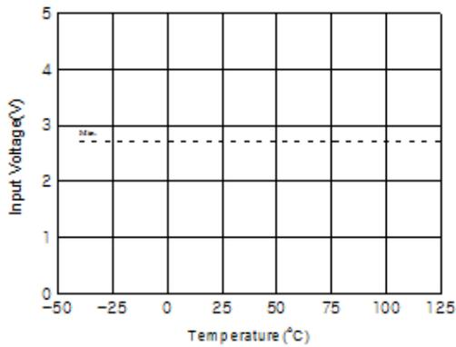
Figure 31. Logic Low Input Voltage vs. Temperature
