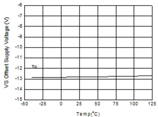
**Figure 62. Maximum vs. Negative Offset Voltage vs. Temperature**
