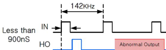
Figure 6. Abnormal Output Waveform with Pulse Width
