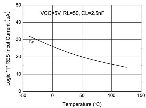
Figure 9. Logic "1" RESET Input Current vs Temperature
