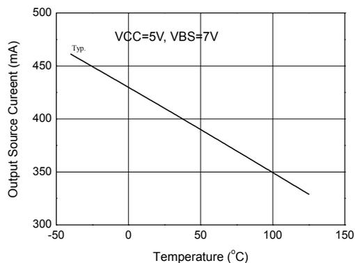
Figure 5b. Output Source Current vs Temperature
