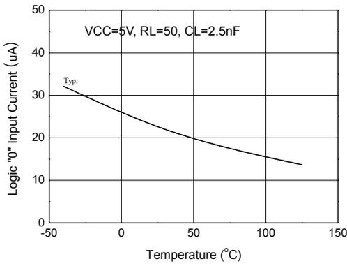
Figure 8. Logic "0" IN Input Current vs Temperature
