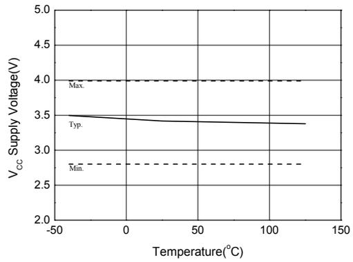
Figure 11b. VCC Under Voltage Threshold(-) vs Temperature
