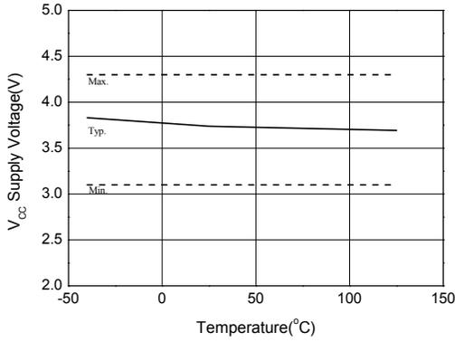
Figure 11a. VCC Under Voltage Threshold(+) vs Temperature
