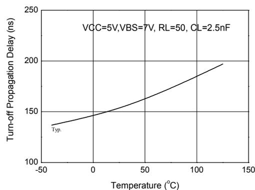
Figure 6b. Turn-Off Propagation Delay Time vs Temperature
