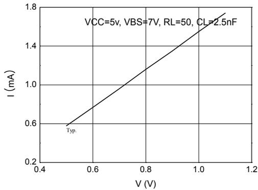
Figure 14. Recharge FET I-V curve
