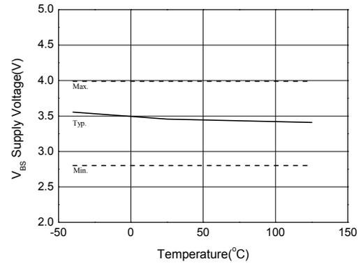
Figure 10b. VBS Under Voltage Threshold(-) vs Temperature
