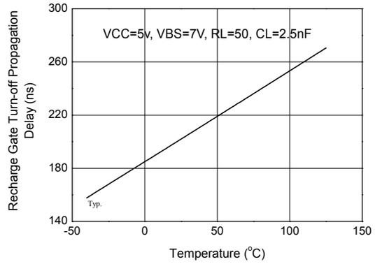
Figure 12. Recharge FET Turn-off Delay time
