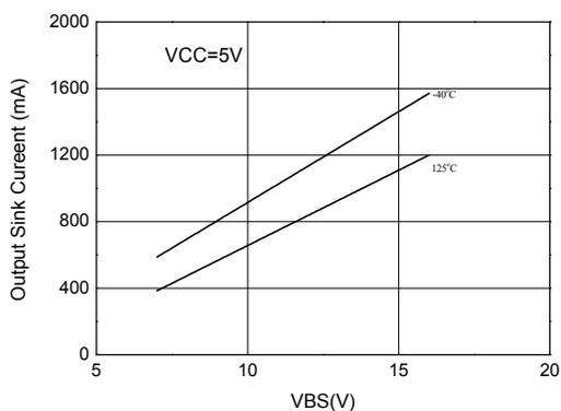
Figure 5a. Output Sink Current vs VBS Supply
