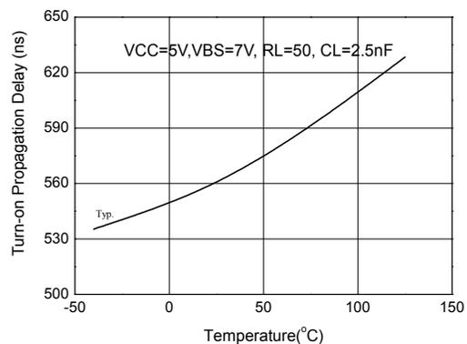
Figure 6a. Turn-On Propagation Delay Time vs Temperature
