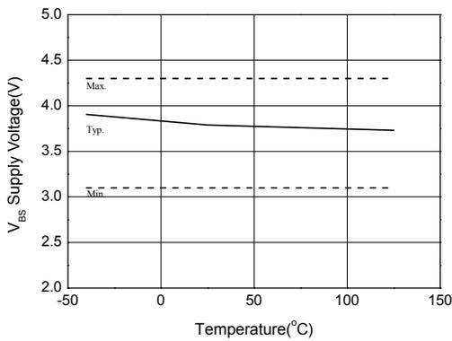
Figure 10a. VBS Under Voltage Threshold(+) vs Temperature
