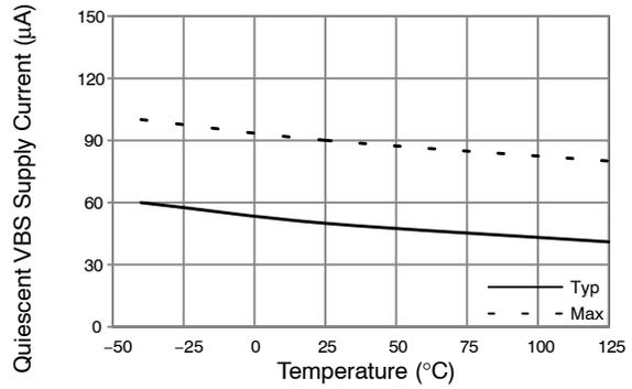
Figure 13. Quiescent  $V_{BS}$  Supply Current vs. Temperature
