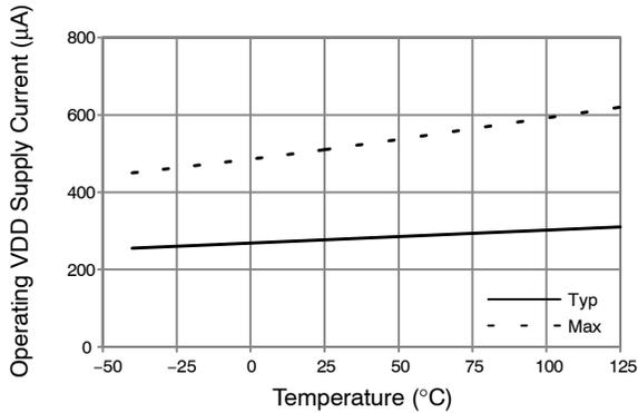
Figure 14. Operating  $V_{DD}$  Supply Current vs. Temperature
