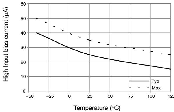
Figure 24. Logic "1" Input Bias Current vs. Temperature
