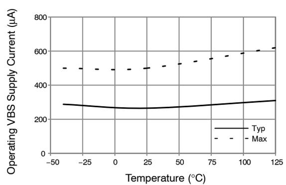
Figure 15. Operating  $V_{BS}$  Supply Current vs. Temperature
