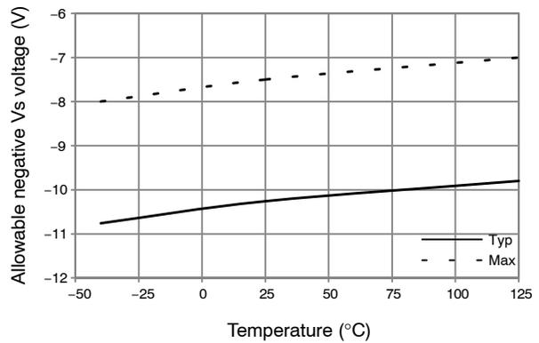
Figure 25. Allowable Negative VS Voltage vs. Temperature
