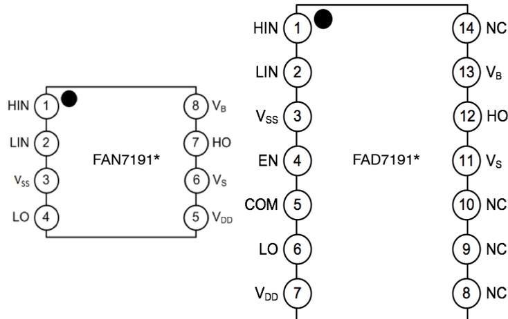
Figure 5. Pin Assignments (Top View)
