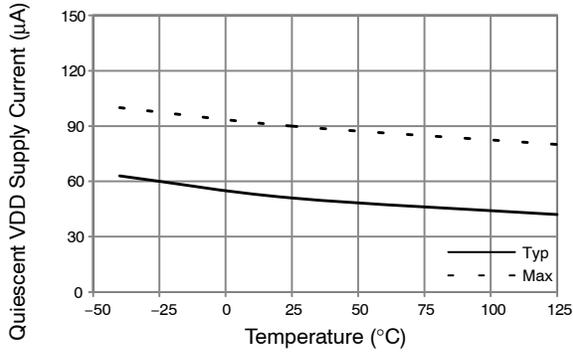
Figure 12. Quiescent  $V_{DD}$  Supply Current vs. Temperature
