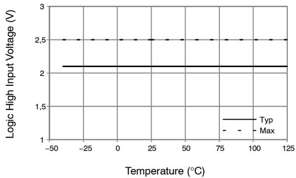
Figure 22. Logic High Input Voltage vs. Temperature
