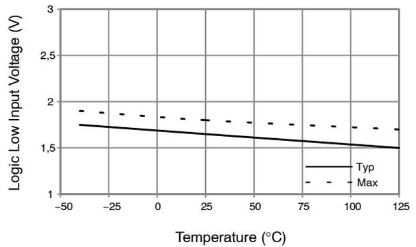
Figure 23. Logic Low Input Voltage vs. Temperature
