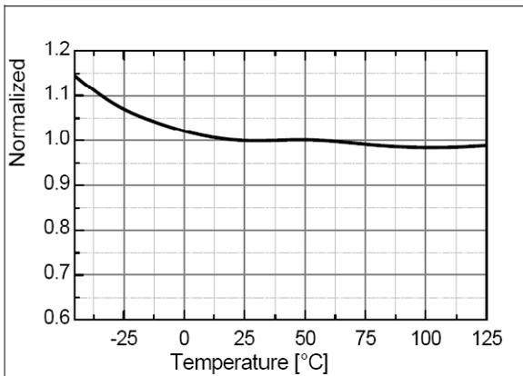
Figure 18. Restart Timer Delay (t<sub>RST</sub>) vs. T<sub>A</sub>
