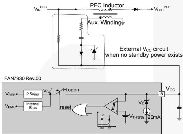
Figure 22. Startup Circuit
