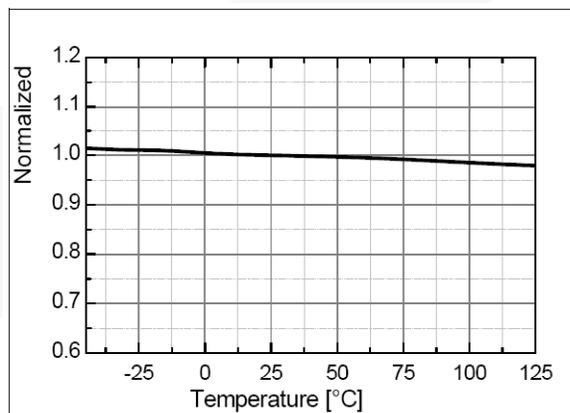
**Figure 9. Output Upper Clamp Voltage (V<sub>EAH</sub>) vs. T<sub>A</sub>**
