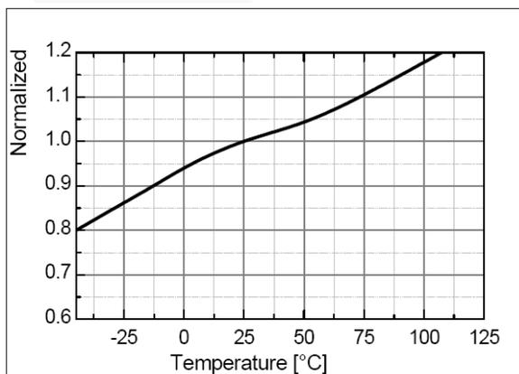
Figure 20. Output Saturation Voltage (V<sub>RDY,SAT</sub>) vs. T<sub>A</sub>
