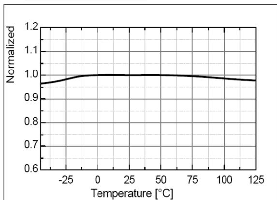
**Figure 8. Operating Supply Current (I<sub>OP</sub>) vs. T<sub>A</sub>**
