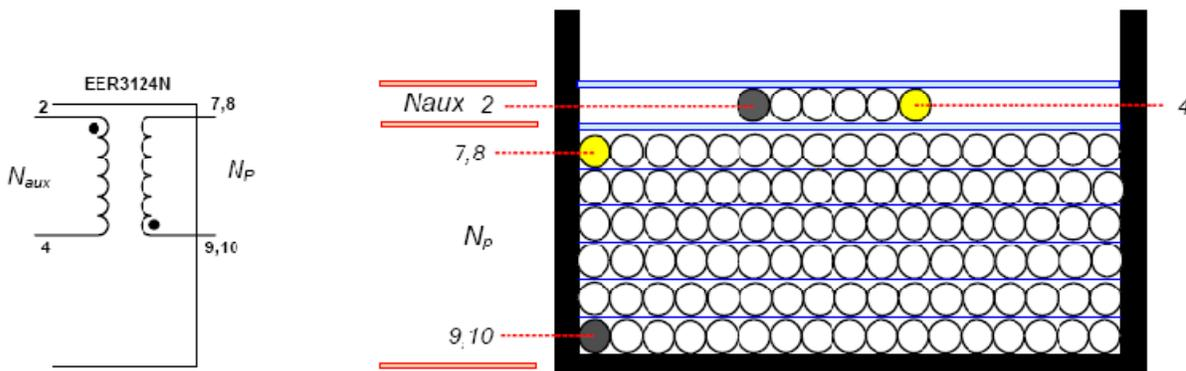
Figure 46. Transformer Schematic Diagram
