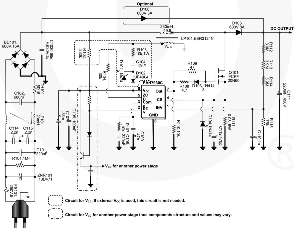
Figure 45. Demonstration Circuit
