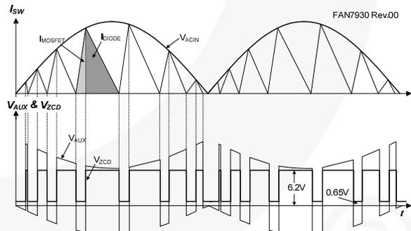
**Figure 28. Auxiliary Voltage Depends on MOSFET Switching**
