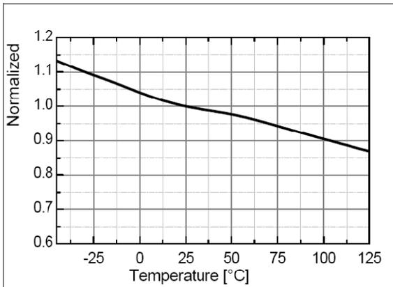
**Figure 7. Startup Supply Current (I<sub>START</sub>) vs. T<sub>A</sub>**
