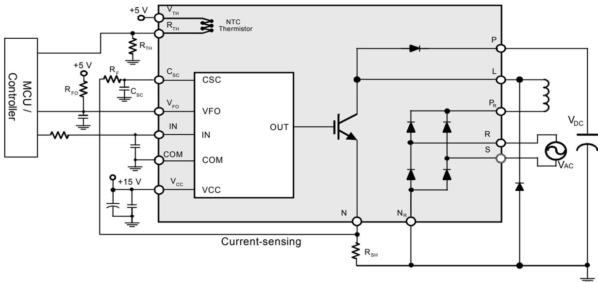
**Figure 9. Typical Application Circuit**
