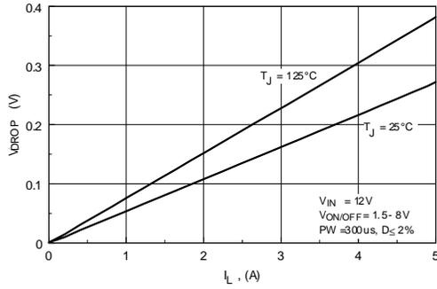
**Figure 1. Conduction Voltage Drop Variation with Load Current.**
