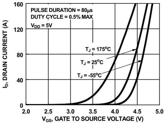
Figure 7. Transfer Characteristics
