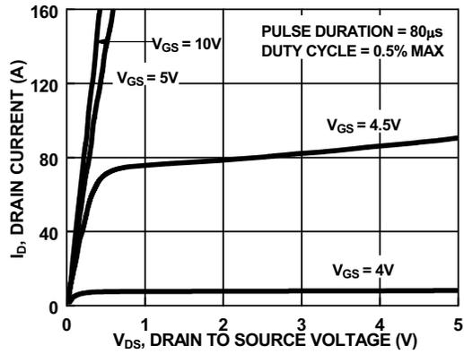
Figure 8. Saturation Characteristics
