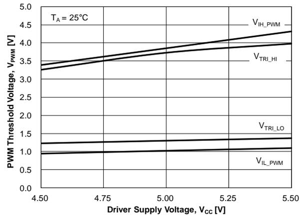
Figure 16. PWM Threshold vs. Driver Supply Voltage
