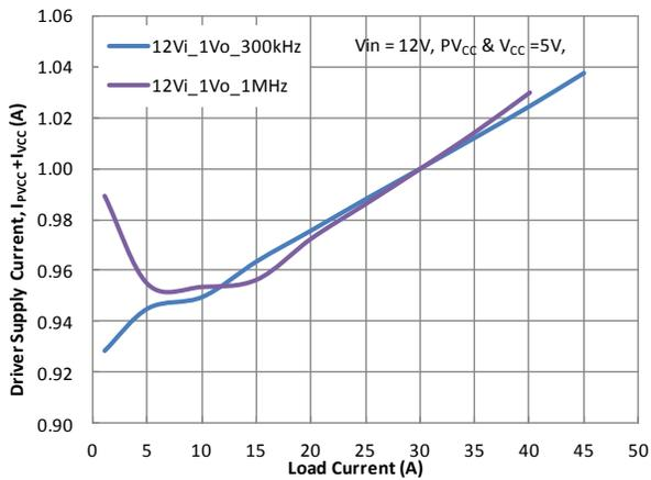
Figure 14. Driver Supply Current vs. Output Current
