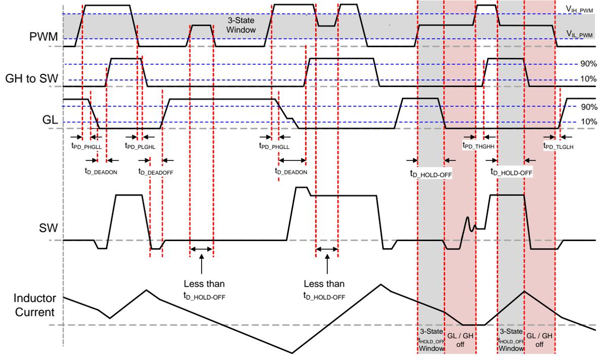
Figure 27. PWM 3-State Timing Diagram (FCCM held HIGH)
