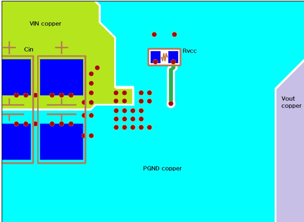
**Figure 31. Single-Phase Board Layout Example – Bottom View (Mirrored)**
