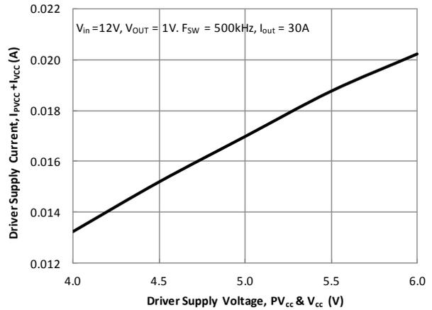
Figure 13. Driver Supply Current vs. Driver Supply Voltage
