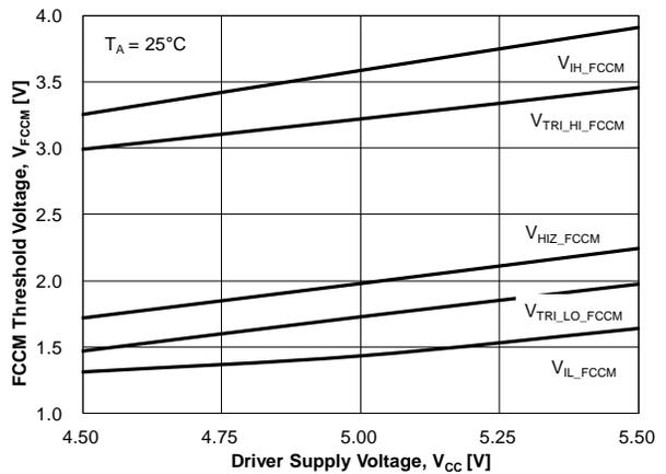
Figure 18. FCCM Threshold vs. Driver Supply Voltage
