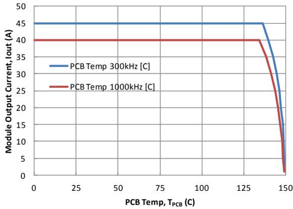
**Figure 4. Safe Operating Area with 12 V<sub>IN</sub>**
