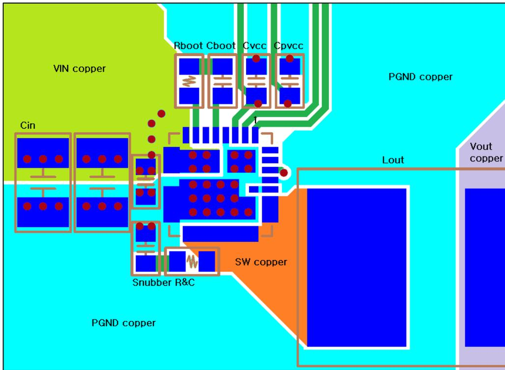
**Figure 30. Single-Phase Board Layout Example – Top View**
