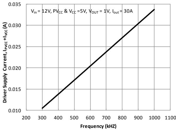
Figure 12. Driver Supply Current vs. Switching Frequency
