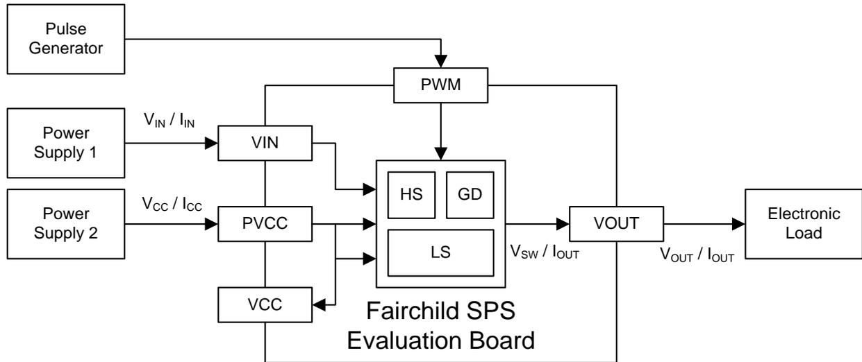
Figure 29. Power Loss and Efficiency Measurement Diagram
