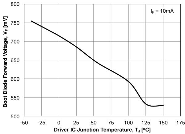
**Figure 21. Boot Diode Forward Voltage vs. Temperature**
