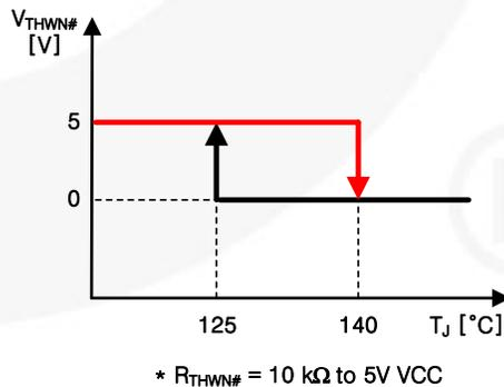
Figure 35. Gate Driver  $T_J$  vs.  $V_{THWN\#}$
