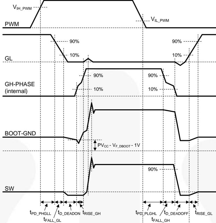
$t_{PD\_PHGLL}$  = PWM HI to GL LO,  $V_{IH\_PWM}$  to 90% GL
