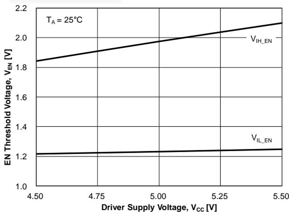
Figure 20. EN Threshold vs. Driver Supply Voltage
