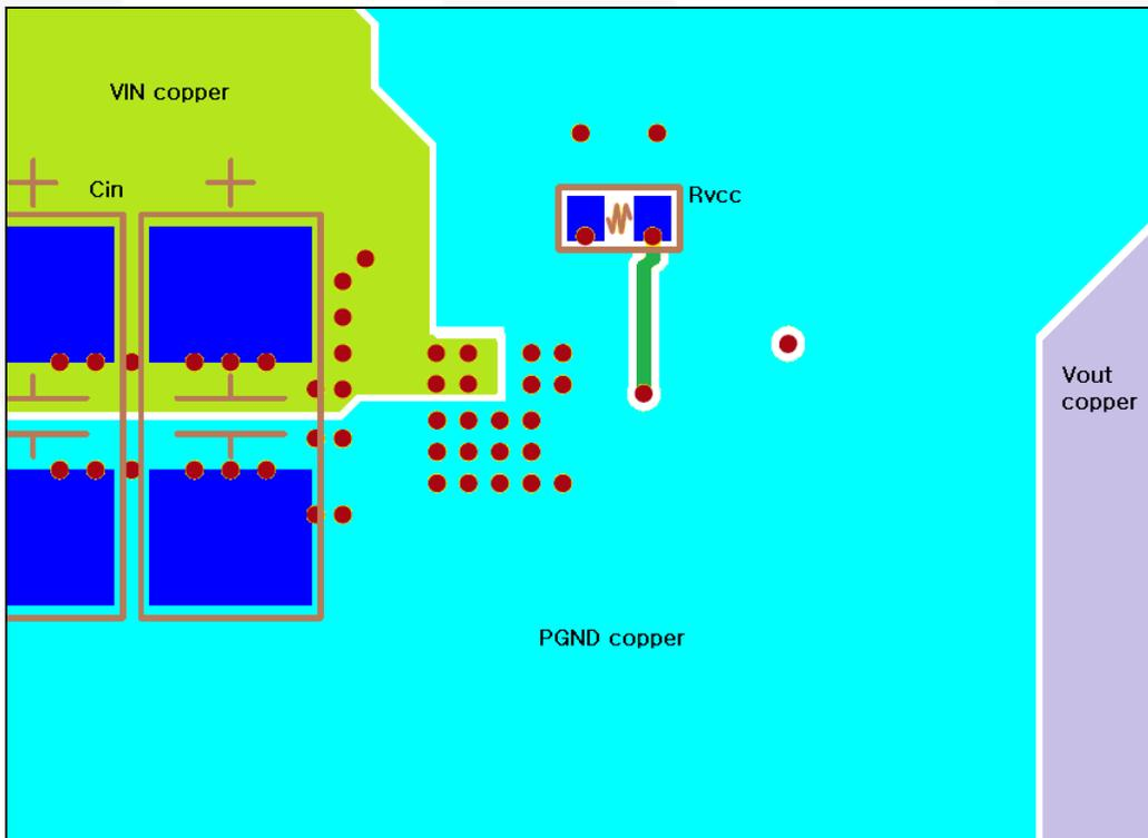
**Figure 39. Single-Phase Board Layout Example – Bottom View (Mirrored)**
