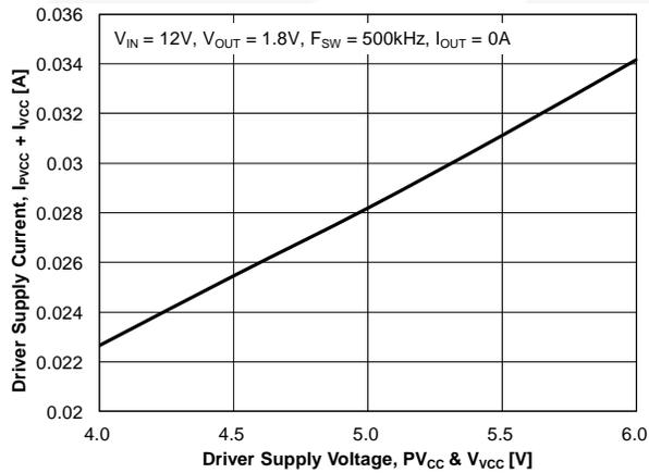
Figure 12. Driver Supply Current vs. Driver Supply Voltage
