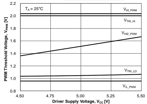
Figure 15. PWM Threshold vs. Driver Supply Voltage
