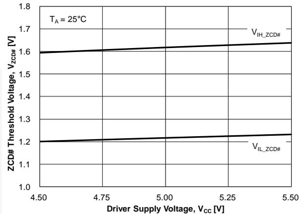
Figure 17. ZCD# Threshold vs. Driver Supply Voltage
