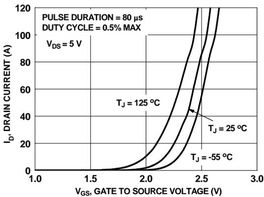
Figure 18. Transfer Characteristics
