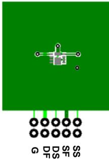
a. 77 °C/W when mounted on a 1 in<sup>2</sup> pad of 2 oz copper
