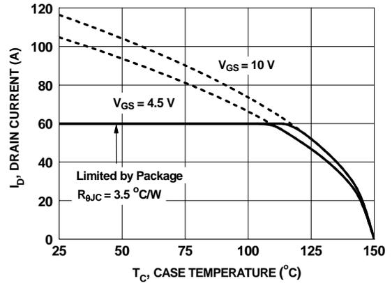
**Figure 23. Maximum Continuous Drain Current vs Ambient Temperature**
