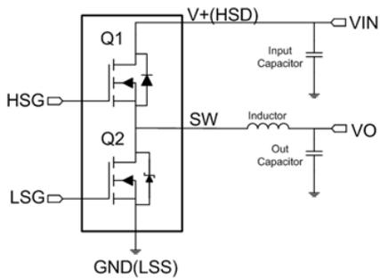
**Figure 1. Power Clip in Buck Converter Topology**
