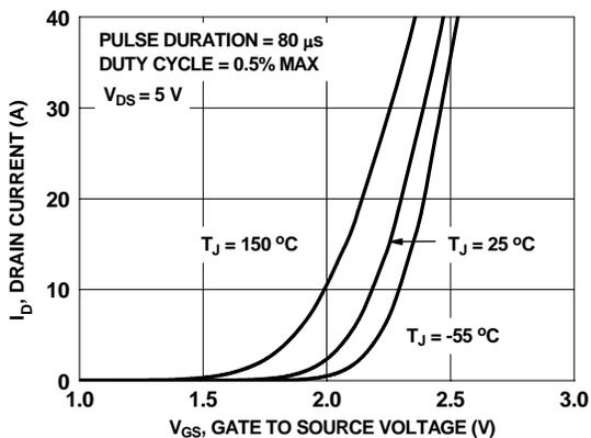
Figure 5. Transfer Characteristics
