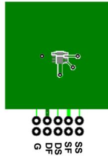
b. 63 °C/W when mounted on a 1 in<sup>2</sup> pad of 2 oz copper
