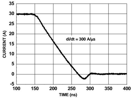
Figure 27. FDPC8011S SyncFET™ body diode reverse recovery characteristic
