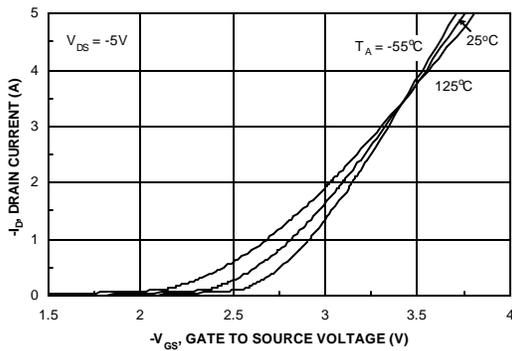
Figure 5. Transfer Characteristics.
