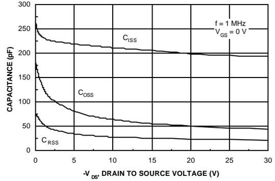
Figure 8. Capacitance Characteristics.
