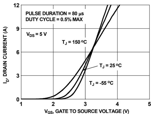
**Figure 5. Transfer Characteristics**
