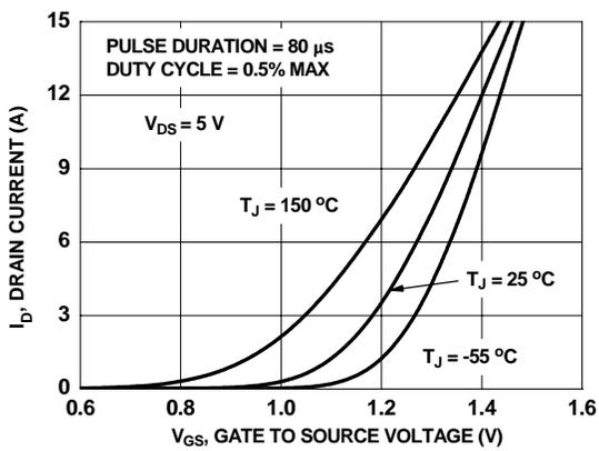
**Figure 5. Transfer Characteristics**
