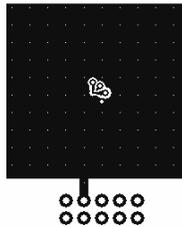
a. 65  $^\circ\text{C}/\text{W}$  when mounted on a 1 in<sup>2</sup> pad of 2 oz copper.
