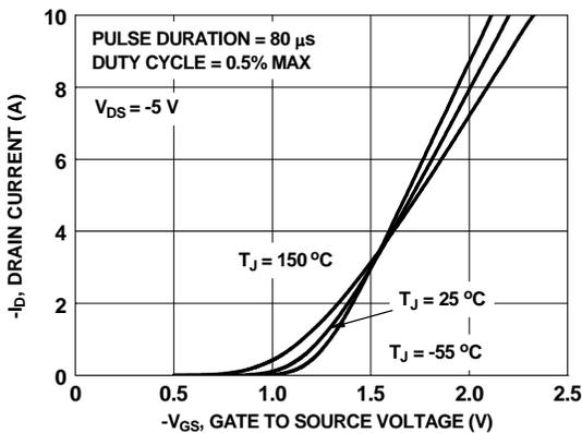
Figure 5. Transfer Characteristics
