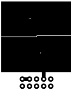
a.  $93\text{ }^\circ\text{C/W}$  when mounted on a  $1\text{ in}^2$  pad of 2 oz copper.
