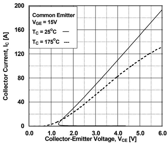
**Figure 4. Transfer Characteristics**
