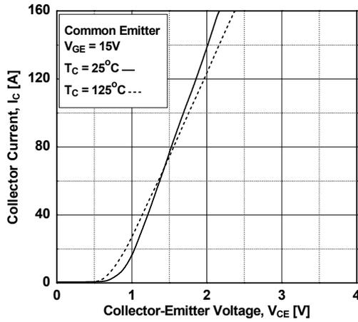
Figure 4. Transfer Characteristics
