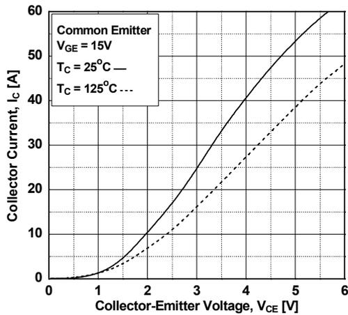
**Figure 4. Transfer Characteristics**
