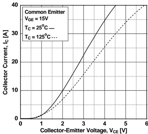
Figure 4. Transfer Characteristics
