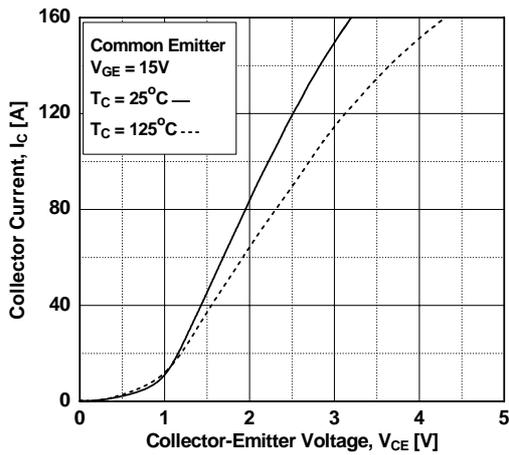
Figure 4. Transfer Characteristics
