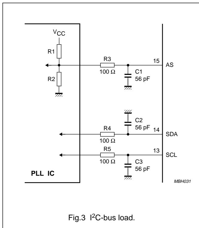
Fig.3 I<sup>2</sup>C-bus load.
