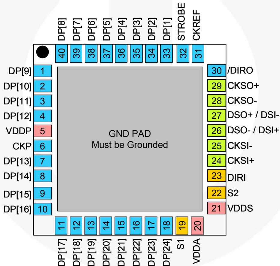
Figure 2. MLP-40 Pinout (Through View)
