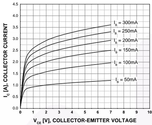
Figure 1. Static Characteristic
