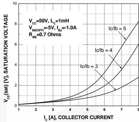
**Figure 8. Collector- Emitter Saturation Voltage at RBSOA**
